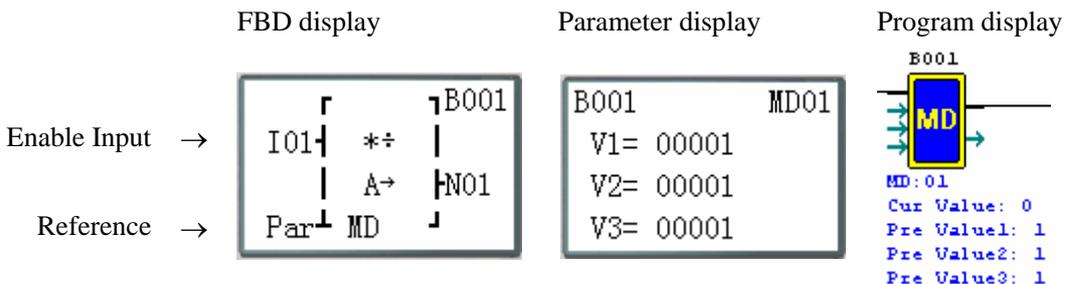
**PID (Proportion- Integral- Differential) function block**
