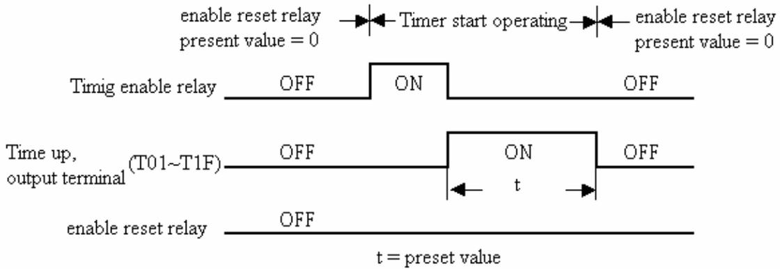
※ T0E and T0F keep their current value after a loss of power to the smart relay if “M Keep” is active, but the others’ reset to 0.
