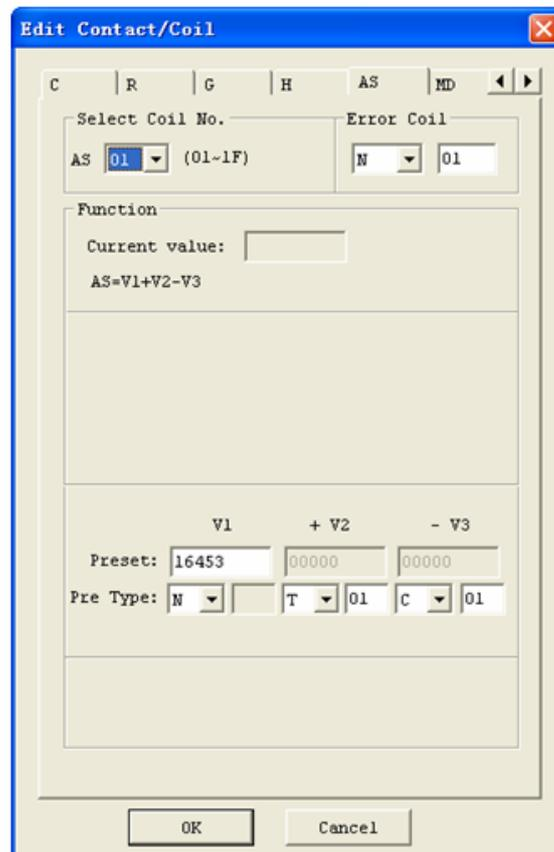
✘ Error output coil N01 will turn ON when the compute result is overflow.
