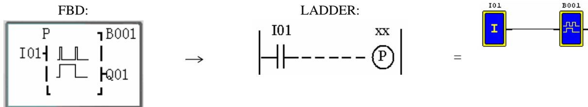
Note: The input terminal is NOP which is equivalent to “Lo”
