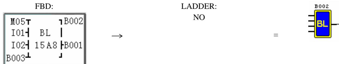
Note: The input terminal is NOP which is equivalent to “Lo”
