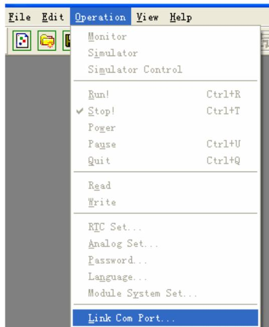
c. Select the correct Com Port number where the programming cable is connected to the computer then press the “Link” button.
