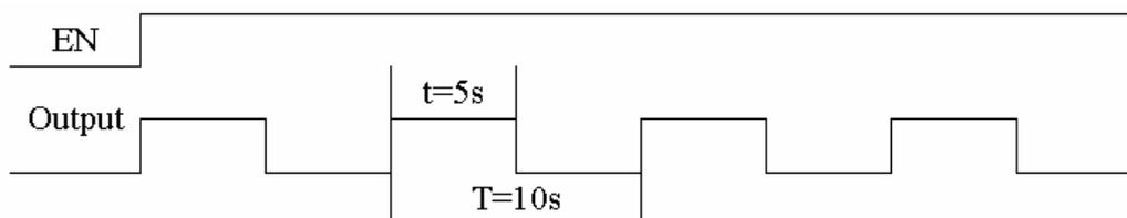
The state of M01, M02 and M03 decide PWM output. PWM stages can be changed by the status of M01, M02 and M03 when P01 is running. ⑥ displays the number of pulse when P01 is running, but ⑥ equals 0 when P01 is disabled.
