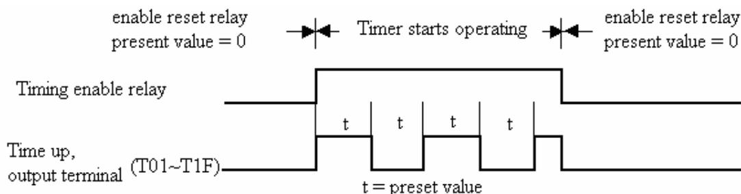
※ The current value of Timer can not be kept on a loss of power to smart.
