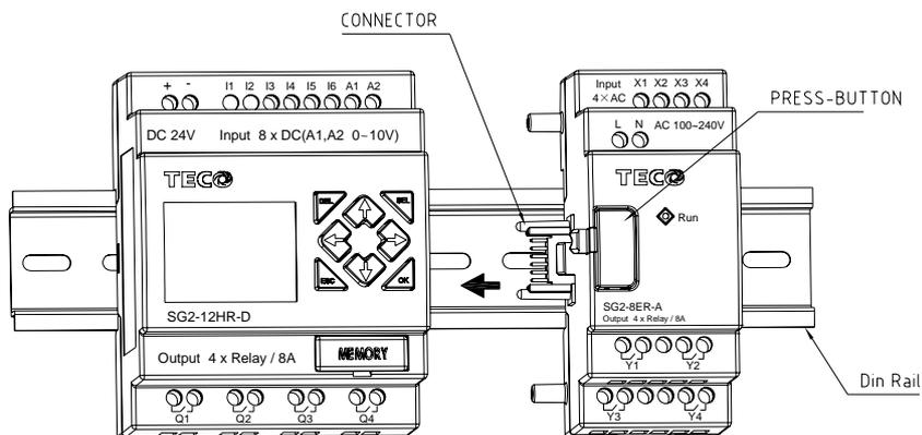
It is recommended to apply a DIN-rail end clamp to hold the SG2 in place.
