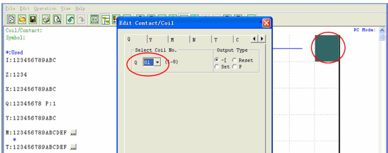
d. Test the simple program. From the Operation menu, select the Write function and write the program to the connected smart relay as shown below.
