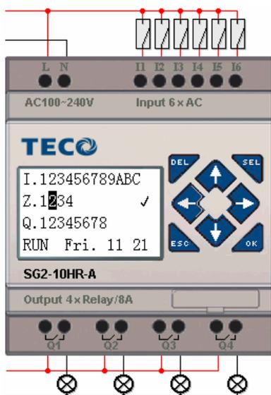
Press "←" (Z02) to disable H03 coil, and the LCD display changes to initial frame.
