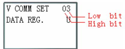
The two bits of keypad how to decide the communication format and baud rate like describing below.
