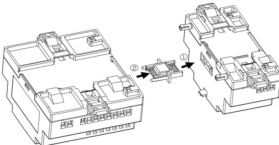
※ The method of all expansion modules connecting with SG2 is the same as shown above.
