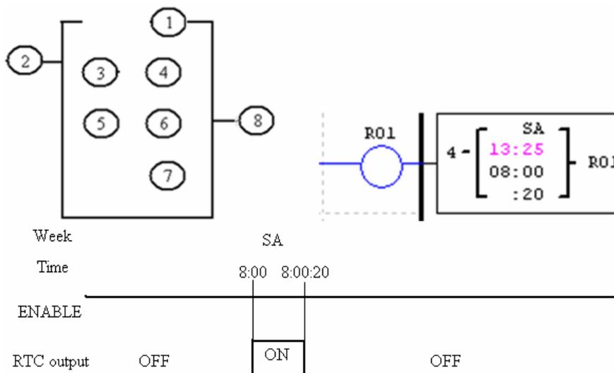
※ The present time will be 8:00:00 when it achieves 8:00:20 at first time, and RTC status bit R01 will be ON. RTC status bit R01 will be OFF when the present time achieves 8:00:20 at second time. Then time continuous going. So, this means that RTC status bit is ON for 21 seconds.
