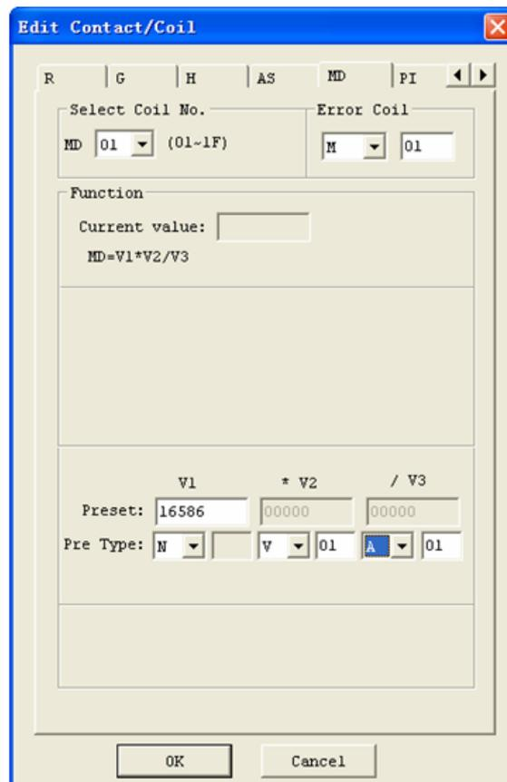
※ Error output coil M01 will turn ON when the compute result is overflow.
