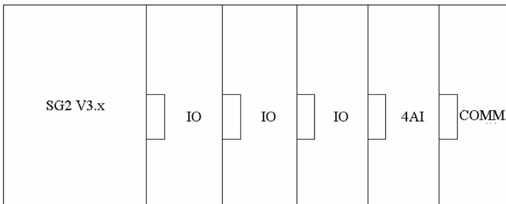
※ digital IO: SG2-8ER-A, SG2-8ER-D, SG2-8ET-D, SG2-8ER-24A
