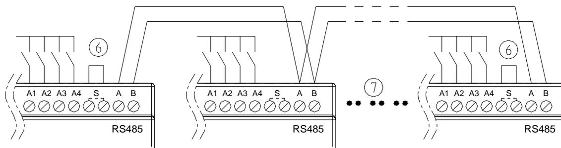
The power supply and the I/O supply should share the same power source. Only short circuit the first and the last module.
