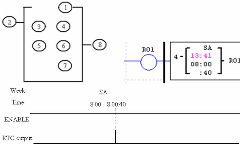
✘ The present time will change to be 8:01:00 when it achieves 8:00:40, and RTC status bit R01 turns ON. Then time is going on and R01 turns OFF. This means that the RTC status bit will be ON for one pulse.
