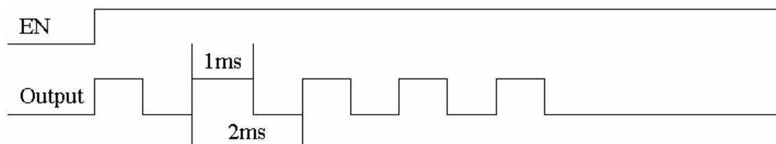
PLSY stops outputting when the number of output pulse is completed.
