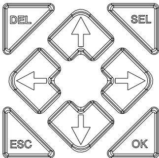
Select (SEL) – Used to select the available memory and instruction types for editing. Holding the Select button will display all “H” HMI/Text messages on the LCD.
