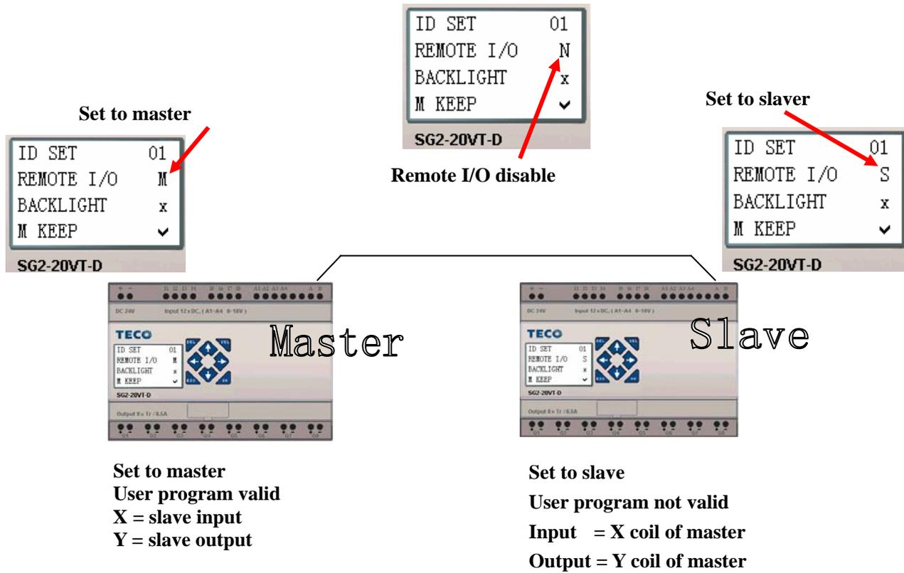
Don't use expansion DI/DO modules, when remote I/O function is enabled.
