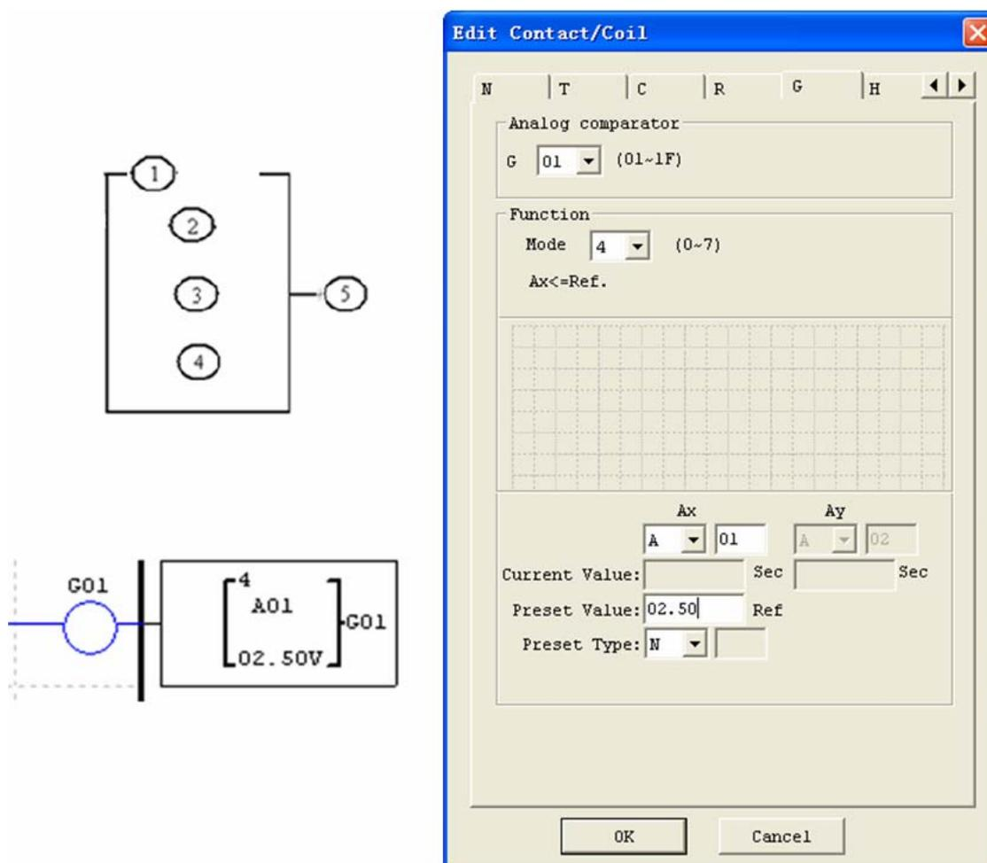
The figure illustrates the configuration of an analog comparator. On the left, a schematic shows a vertical stack of four terminals labeled 1, 2, 3, and 4. Terminal 1 is connected to terminal 5. Below this, a ladder logic diagram shows a coil labeled G01 connected to a contact block. The contact block contains a mode selector '4', the input 'A01', and a preset value '02.50V'. The output of the contact block is also labeled G01.
