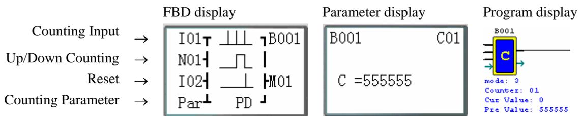
Note: The "PD" means the current value will be retain until the power recover; Counter keeps current value when the smart switches between RUN and STOP when C KEEP enable;
