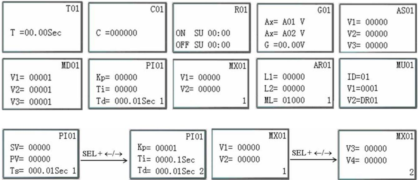
Under FBD mode, Press “SEL” key, Block displays in sequence.
