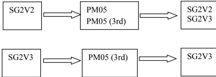
The optional PM05 (3rd) memory cartridge is used to easily transfer programs from one smart relay to another. The PM05 (3rd) memory cartridge plugs into the same connector as the programming cable (see procedure below).
