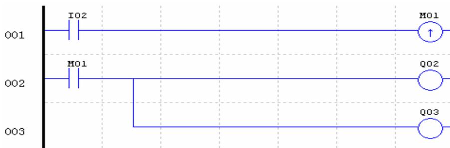
※ The state of auxiliary relays “M01~M3F” will be kept when the smart powers down if “M Keep” is active. “M Keep” can be set by the two ways below.
