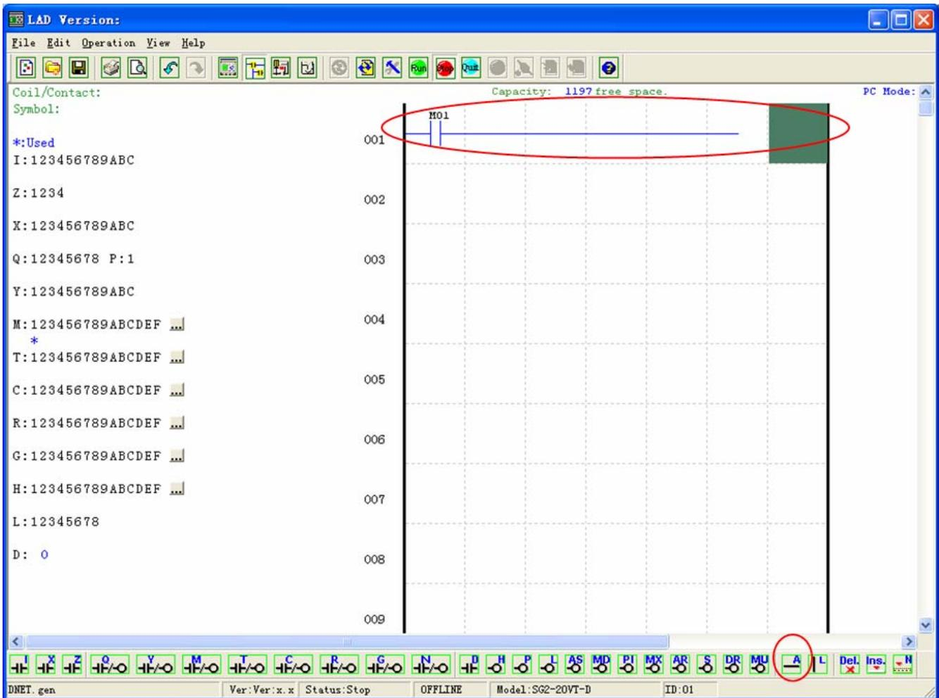
c. Select the “Q” coil icon from the ladder toolbar and drop it on the right most cells. Select Q01 from the dialog and press OK as shown below. See Chapter 4: Ladder Programming instructions for complete instruction set definitions.
