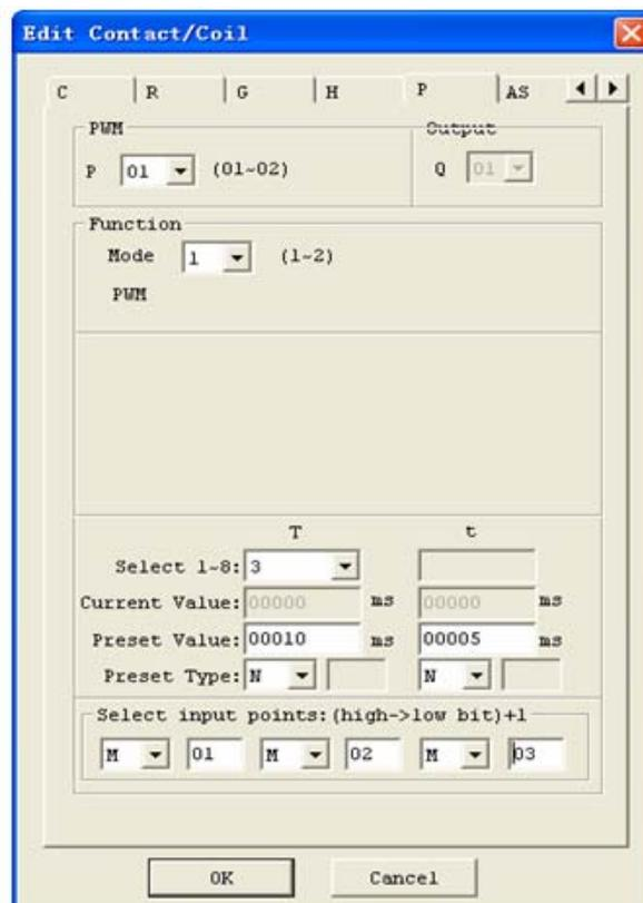
The state of M01, M02 and M03 are 010, so PWM output pulse is like this as setting above:
