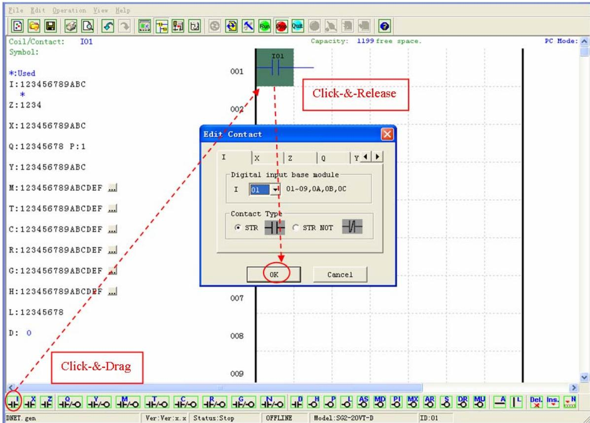
The “A” and “L” keys or icons are used to complete parallel and serial circuits. The right column is for output coils.
