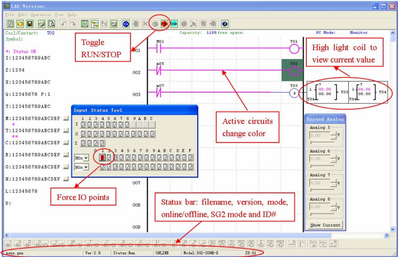
※ The SG2 Client software does not support runtime logic editing changes. All logic edits to contacts, coils, Timers/Counters, and circuit connecting lines must be written to the connected smart relay while in Stop mode.
