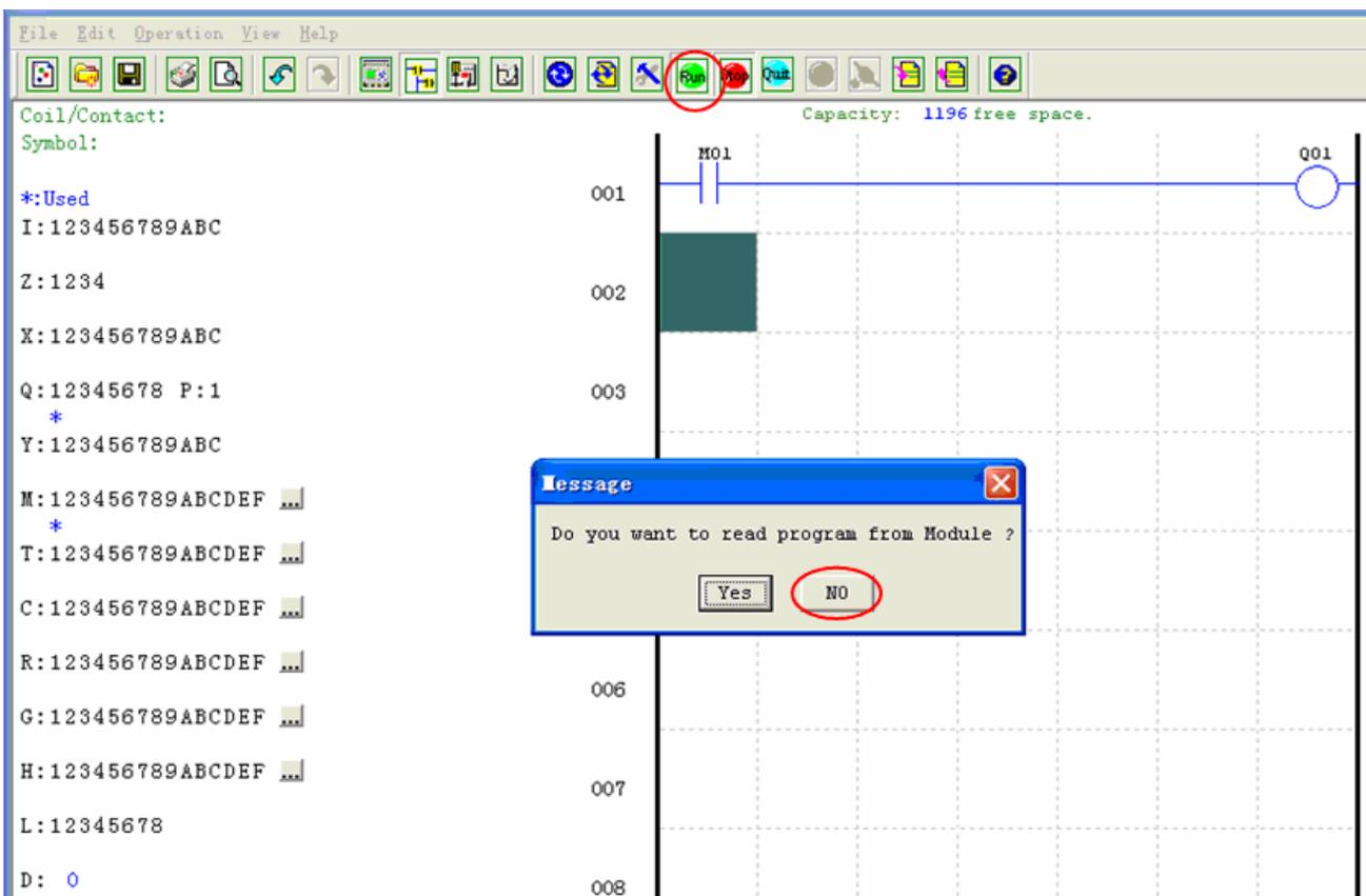
f. On the Input Status dialog, click on M01 to activate the contact M01 which will turn ON the Output Q01 as shown below. The highlighted circuit will show active and the first Output (Q01) on the connected smart relay will be ON. See Chapter 3: Programming Tools for more detailed software information.
