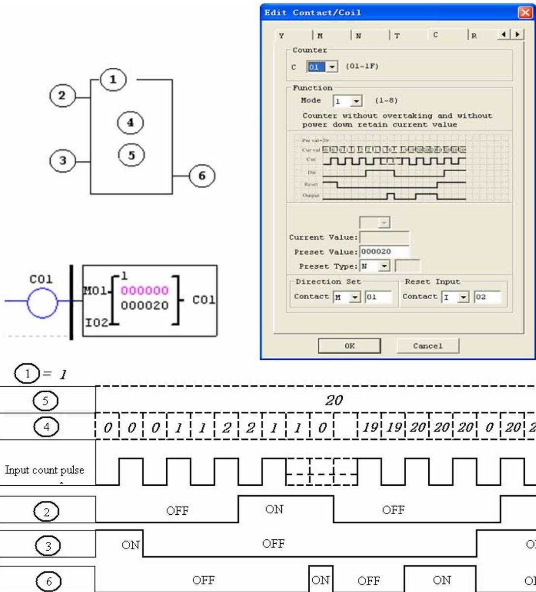
✘ Under this mode, the counter current value will be init value when the smart is power up or switching between RUN and STOP. The init value is 0 if the counter configured as counting up, else, it is preset value.
