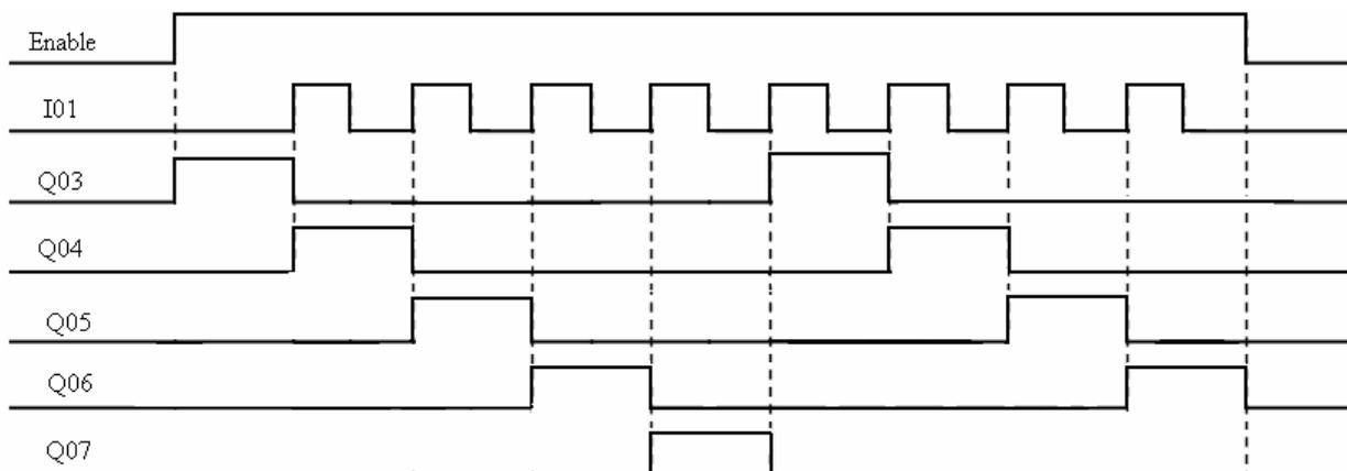
※ Q03 is ON, and from Q04 TO Q07 are OFF when ENABLE is active. Q04 turns ON when I01's rising edge coming on, and others points turn OFF. The next coil turns ON at each rising edge of SHIFT input, and others turn OFF.
