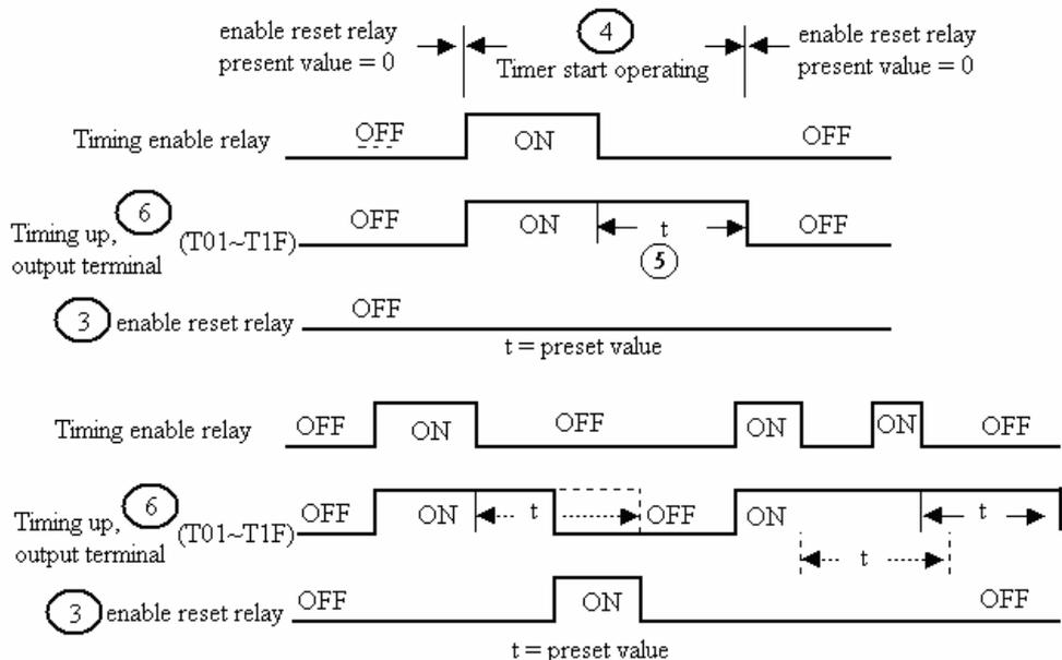
※ T0E and T0F keep their current value after a loss of power to the smart relay if “M Keep” is active, but the others’ reset to 0.
