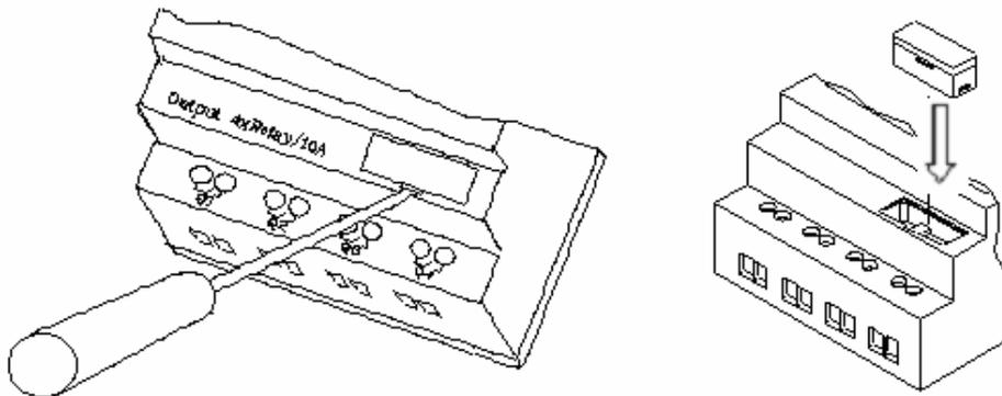
3. From the display keypad on the face of the SG2 smart relay, select either **WRITE** or **READ** to transfer the program to PM05 (3rd) or from the PM05 (3rd) memory cartridge to the smart relay.
