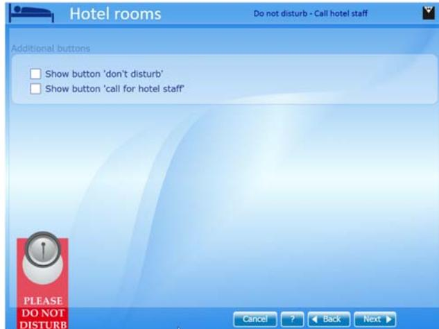
Select the two checkboxes and the "Do not disturb" and "Room service" buttons are shown on the page being created :
