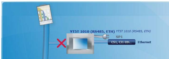
On the "Device connection management" page, your YT5T device still has a serial port (SP1 port) available. You add a serial protocol by simply clicking the drop-down menu shown below and select the "Serial" communication standard :
