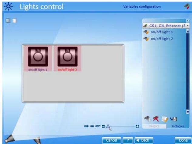
You will notice the objects on the page are pink in colour. This means they have not yet been assigned a variable. The first thing to do, therefore, is to create a variable (see chapter 4, "Creating a new variable" page 53). Create the variable (in the example, "on/off light 1"). Select it with the mouse and drag it onto the selected button :
