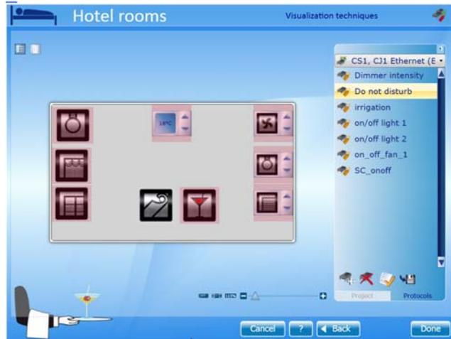
The "Do not disturb" button changes colour. The pink image disappears. You can move the cursor over the button to view the properties of the assigned variable :
