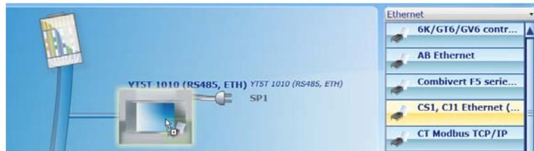
As can be seen below, the protocol appears not in the same way as for the "Local Network", but on the left of the graphical representation of the Ethernet cable :
