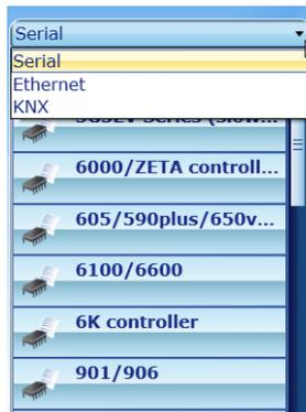
A list appears automatically stating all the "serial" protocols that can be assigned to the ESA device. Select a protocol and drag it (pressing and holding the left button on the mouse) to the ESA device :
