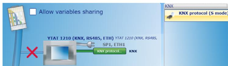
Select the required Konnex protocol and drag it onto the ESA device :
