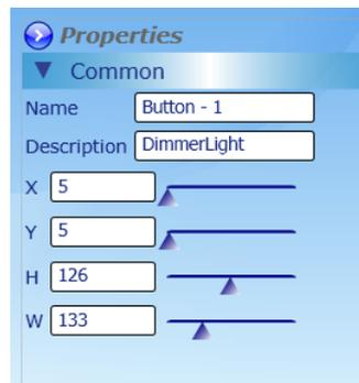
You can also modify the position of the button on the page using the X and Y variables, and edit the width and height of the button using the W and H variables. You can edit the values in the same 3 ways described earlier on :
