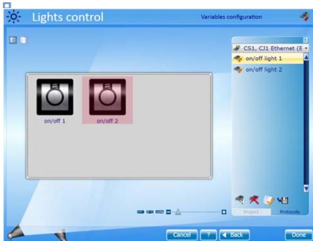
The button changes colour. The pink image disappears. You can move the cursor over the button to view the properties of the assigned variable :
