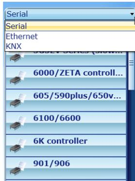
A list appears automatically stating all the "serial" protocols that can be assigned to the ESA device.
