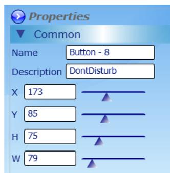
You can also modify the position of the button on the page using the X and Y variables, and edit the width and height of the button using the W and H variables. You can edit the values in the same 3 ways described earlier on :
