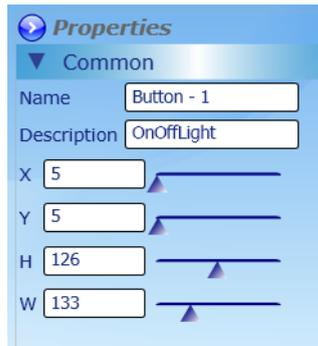
You can also modify the position of the button on the page using the X and Y variables, and edit the width and height of the button using the W and H variables.
