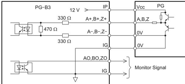
Figure 6 Complementary Outputs for the Interface Circuit
