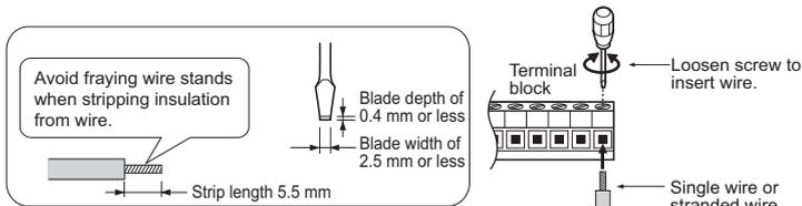
**Figure 11 Terminal Block Wiring**
