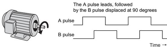
Figure 8 Displacement of A and B Pulses
