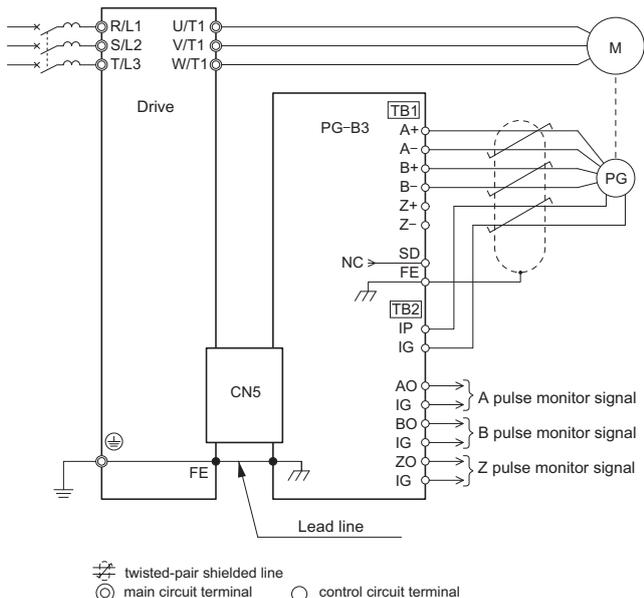
Figure 5 Wiring the Option Card and PG
