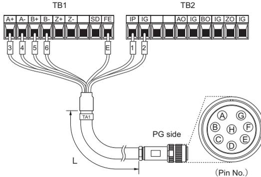
**Figure 9 Wiring PG Cables**
