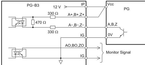
Figure 7 Open-Collector Outputs for the Interface Circuit
