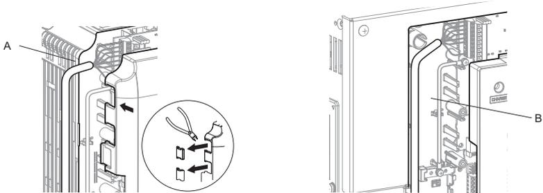
**A** – Wires should pass through the access hold provided on the left side of the front cover.
