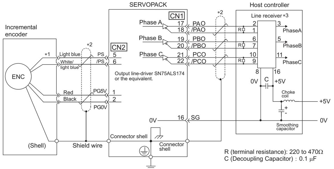
\*1. The pin numbers for the connector wiring differ depending on the servomotors.
