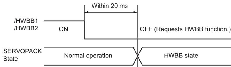
Note: The OFF status is not recognized if the /HWBB1 and /HWBB2 signals are 0.5 ms or shorter.
