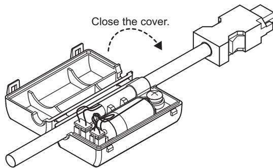
5. After replacing the battery, turn OFF the SERVOPACK power to cancel the absolute encoder battery alarm (A.830).
