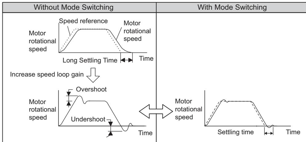
■ Using the Acceleration Level to Switch Modes
