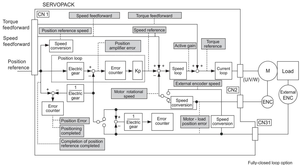
The following signals can be monitored by selecting functions of parameters Pn006 and Pn007. Pn006 is used for analog monitor 1 and Pn007 is used for analog monitor 2.
