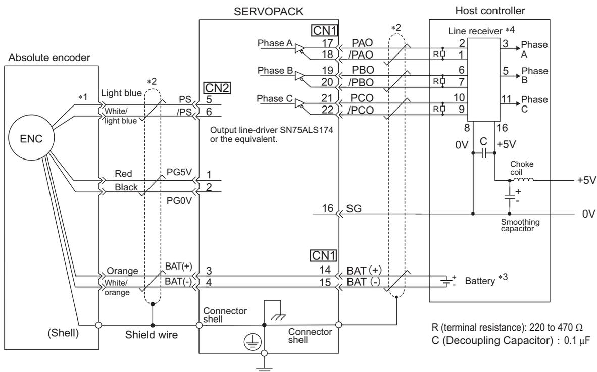
\*1. The pin numbers for the connector wiring differ depending on the servomotors.
