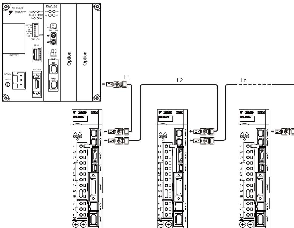
Note: The length of the cable between stations (L1, L2 ... Ln) must be 75 m maximum.
