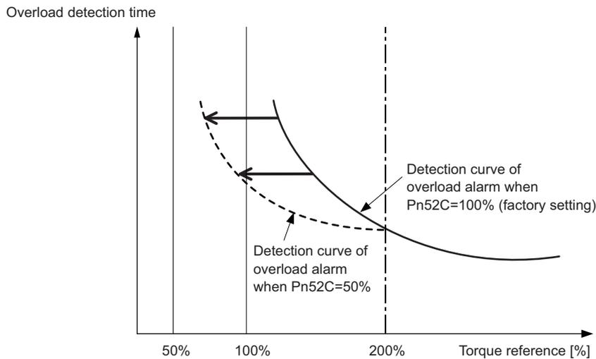
Note: For details, refer to ● *Overload Characteristics* listed in the section for the relevant servomotor in the *Σ-V Series Product Catalog (KAEP S800000 42)*.
