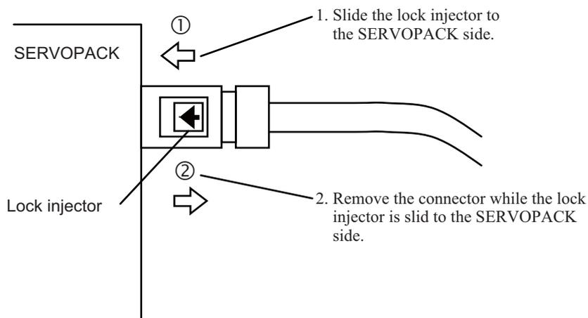
Note: The MECHATROLINK-III communications cable connector may be damaged if it is removed without being unlocking.
