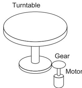
Because the turntable moves in only one direction, the upper limit for revolutions that can be counted by an absolute encoder will eventually be exceeded. The multiturn limit setting is used in cases like this to prevent fractions from being produced by the integral ratio of the motor revolutions and turntable revolutions.
