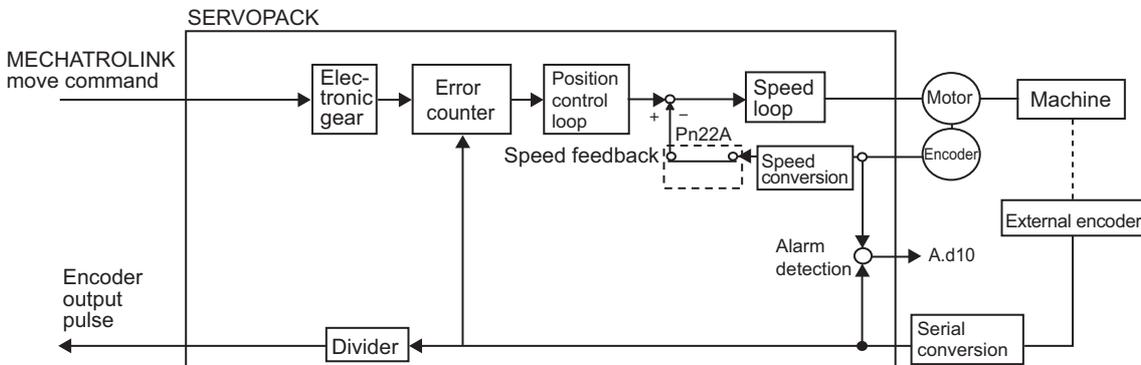
Note: Either an incremental or an absolute encoder can be used. When the absolute encoder is used, set 1 to Pn002.2 (use the absolute encoder as an incremental encoder).
