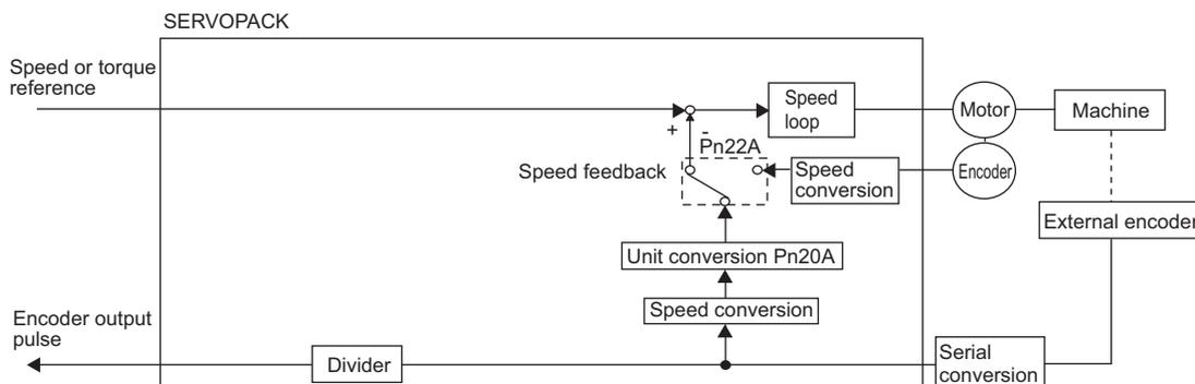
Use Pn22A.3 to select the speed feedback method during fully-closed loop control: Normally, set Pn22A.3 to 0 (Uses motor encoder speed.). Set Pn22A.3 to 1 (Uses external encoder speed.) when connecting a direct drive motor and high-resolution external encoder.
