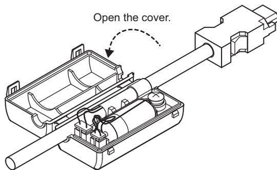
3. Remove the old battery and mount the battery (JZSP-BA01) as shown below.
