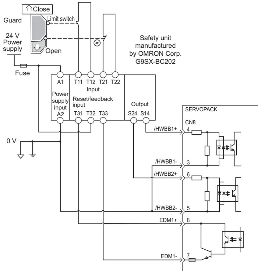
When a guard opens, both of signals, the /HWBB1 and the /HWBB2, turn OFF, and the EDM1 signal is ON. Since the feedback is ON when the guard closes, the safety unit is reset, and the /HWBB1 and the /HWBB2 signals turn ON, and the operation becomes possible.
