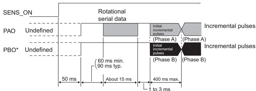
\* In case of reverse rotation mode (Pn000.0 = 1), the output polarity for PBO signal inverts.
