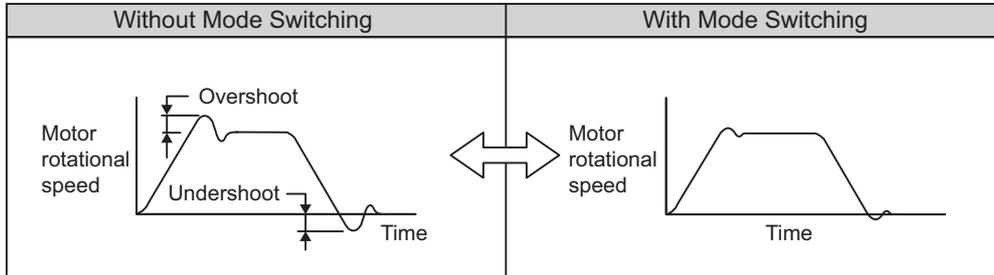
■ Using the Speed Reference Level to Switch Modes
