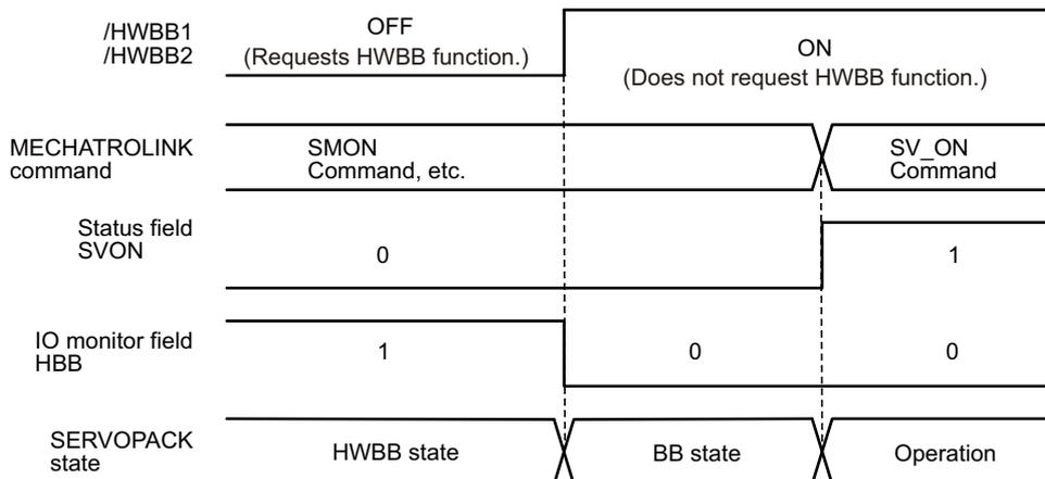
Note: Even if the servomotor power is turned OFF by turning OFF the main circuit power, the HWBB status is retained until a servo OFF command (SV\_OFF: 32 H) is received.
