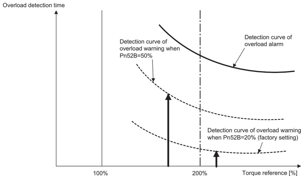
Note: For details, refer to ●Overload Characteristics listed in the section for the relevant servomotor in the  $\Sigma V$  Series Product Catalog (KAEP S800000 42).
