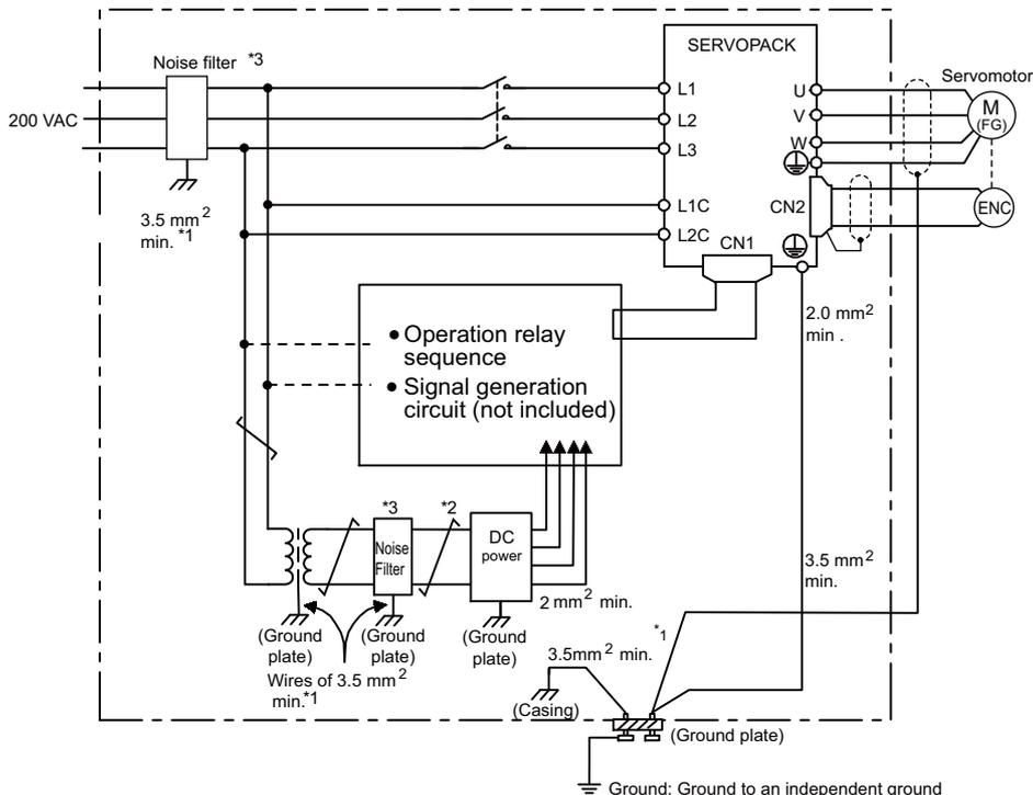
\*1. For ground wires connected to the ground plate, use a thick wire with a thickness of at least 3.5 mm<sup>2</sup> (preferably, plain stitch cooper wire).
