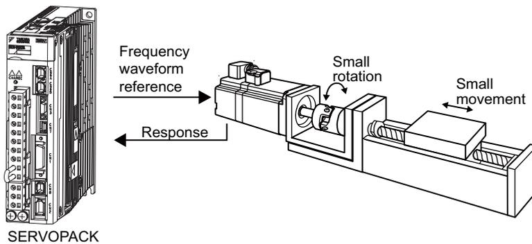
In addition to this function, Online Vibration Monitor (Fn207) can be used to detect machine vibration and automatically make notch filter settings. Use the following flowchart to determine which function should be used.
