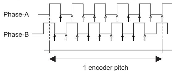
"↑" shows the edge position. In this example, the set value is 20 therefore the number of ↑ is 20.
