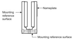
**2.** Place the magnetic way on the reference surface of the machine and secure it with bolts.
