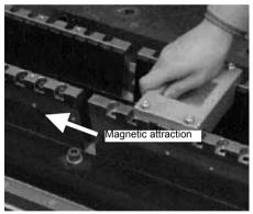
Note: To ensure your safety, install the moving coil before installing second and subsequent magnetic ways. For details, refer to (2) Moving Coil Installation.
