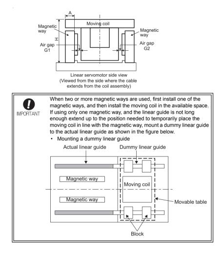
**2.** Insert a thin nonmagnetic (preferably resin) sheet (approximately 0.5mm thick) in the air gap between the moving coil and magnetic way. Then, move the moving coil slowly toward the magnetic way.
