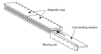
The relationship between the dimensions and positioning between the moving coil's coil winding section and magnetic ways's magnets is shown here. Maintain the following air gaps when installing. Make sure that the moving coil and magnetic way do not interfere with each other during the stroke.
