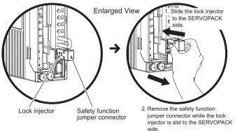
Note: The safety function jumper connector may be damaged if it is removed without being unlocking.
