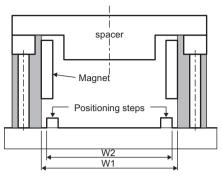
**2.** Insert the mounting bolts into one of the two magnetic way yokes and tighten lightly by hand. Next, while firmly holding down the magnetic way yoke onto the positioning step, tighten the bolts firmly.
