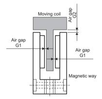
2. Move the moving coil back and forth several times over the magnetic way from end to end, making sure that the moving coil and magnetic way are not touching each other and that no foreign objects such as magnetic particles are present.
