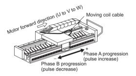
Note: When the direction of the linear servomotor and the direction in which the linear scale counts pulses are reversed because of wiring or other factors, set the parameter Pn080.1=1 (Sets phase B lead as phase sequence of U, V, W).
