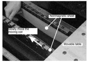
Always be aware of the strong magnetism of the magnetic way and keep fingers and tools at a safe distance, especially when the moving coil is near the magnetic way. The moving coil will be strongly attracted to the magnetic way. When the specified dimensions of the air gaps between the moving coil and the magnetic way are secured, it is not necessary to insert nonmagnetic sheets into the air gaps. (see the table of dimensions in step 1.)
