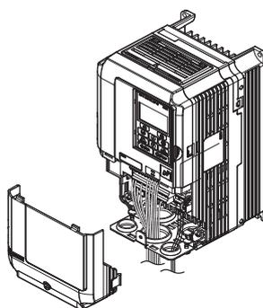
Figure 7.27 Drive Replacement: Removing the Terminal Cover
