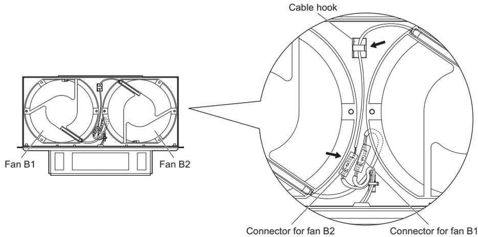
Figure 7.23 Cooling Fan Wiring: 2A0215, 2A0283, and 4A0180
