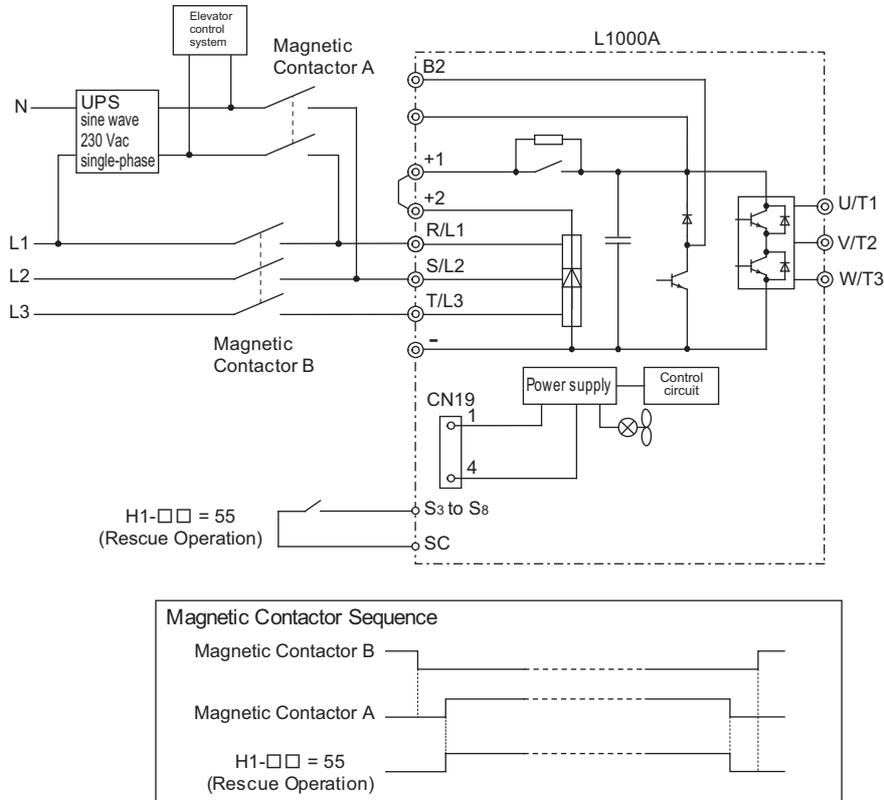
Figure 4.19 Using a Single-Phase 230 V UPS
