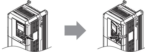
Figure 3.10 Removing the Digital Operator
