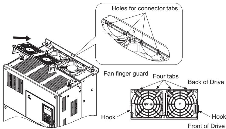
Figure 7.17 Reattach the Fan Cover: 4A0075, 4A0091
