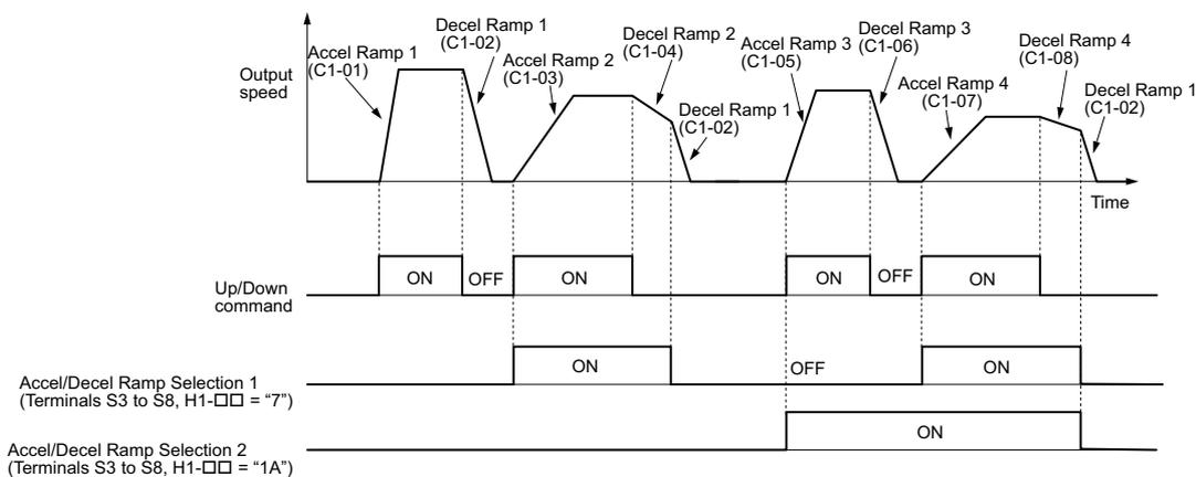
**Figure 5.5 Timing Diagram of Accel/Decel Ramp Change**
