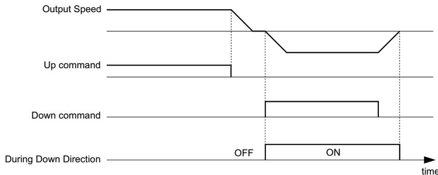
Figure 5.27 Down Direction Output Example Time Chart
