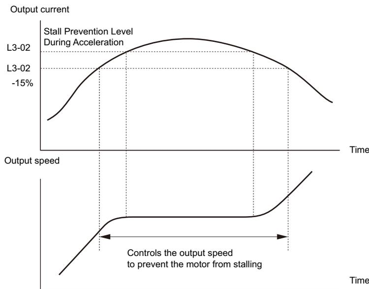
Figure 5.34 Stall Prevention During Acceleration for Induction Motors
