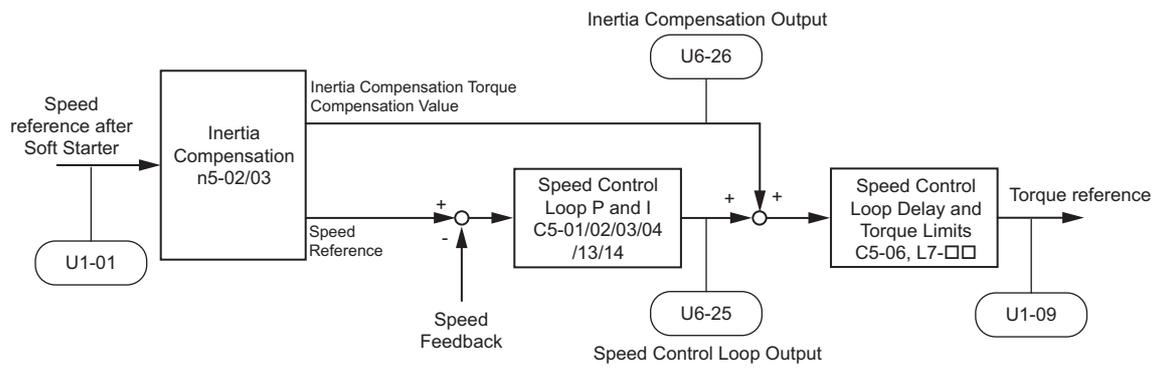
Figure 5.42 Inertia Compensation
