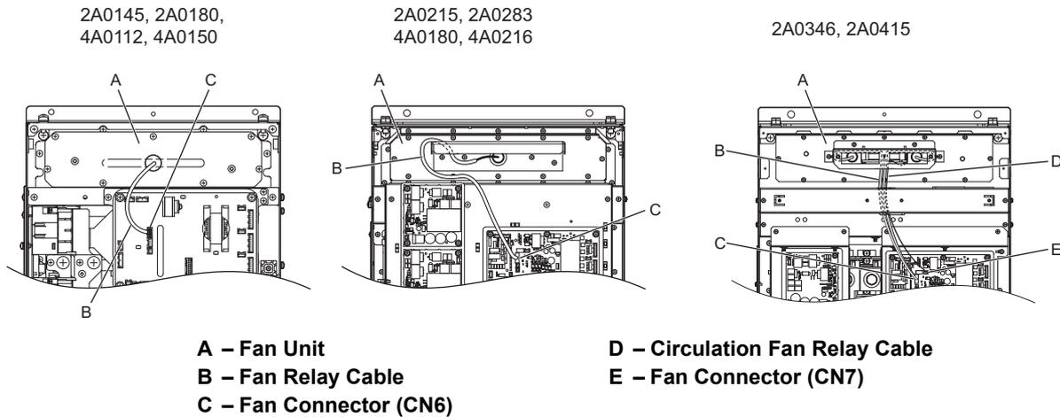
Figure 7.19 Cooling Fan Replacement: Fan Unit and Connectors
