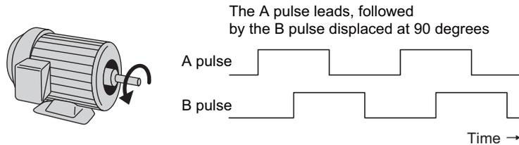
**Figure 8.13 Displacement of A and B Pulses**
