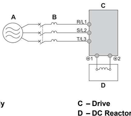
**Figure 8.20** Connecting a DC Reactor
