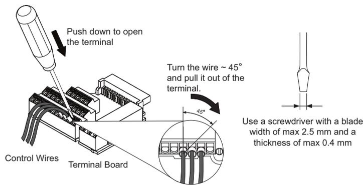
**Figure 3.21 Removing Wires from the Terminal Board**
