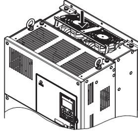
Figure 7.18 Reattach the Fan Cover: 4A0075, 4A0091
