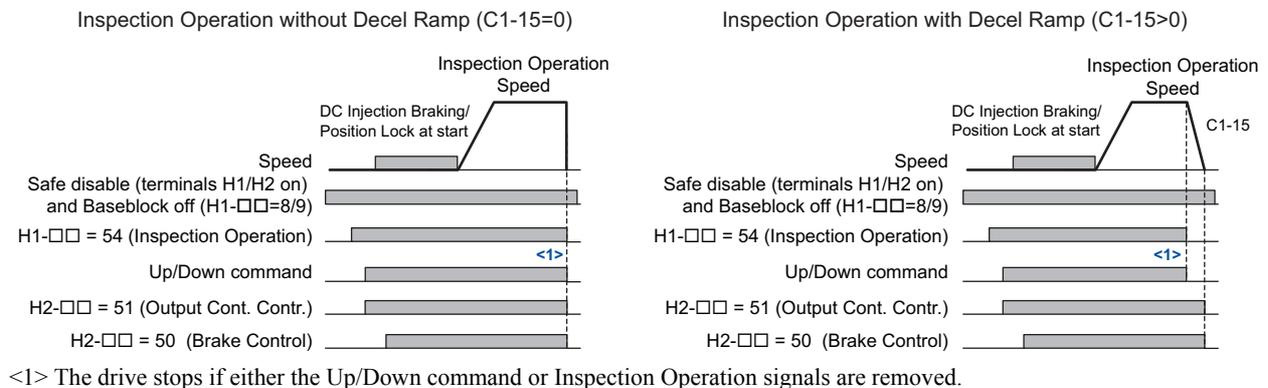
Figure 4.14 Inspection Operation Sequence
