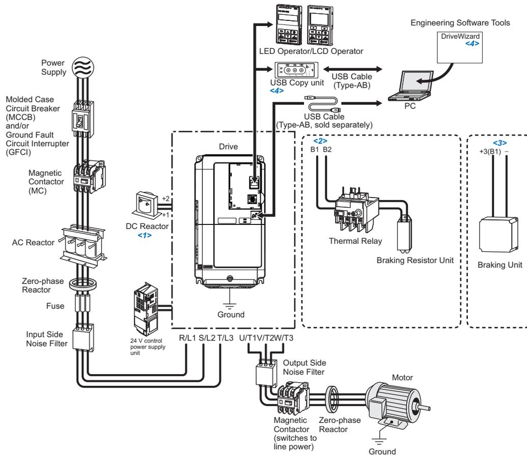
Figure 8.1 Connecting Peripheral Devices
