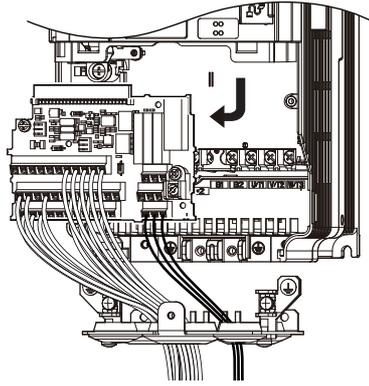
Figure 7.29 Drive Replacement: Remove the Control Terminal Board
