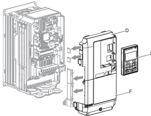
**Figure 8.12 Replace the Front Covers and Digital Operator**
