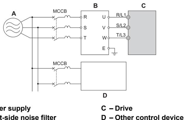
Figure 8.22 Input-Side Noise Filter (Three-Phase 200/400 V)
