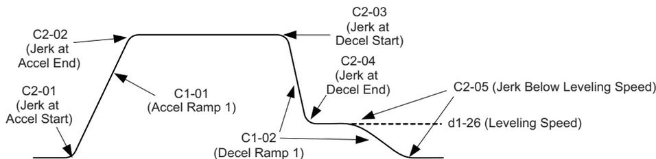
**Figure 4.13 Accel/Decel Ramp and the Jerk Function**
