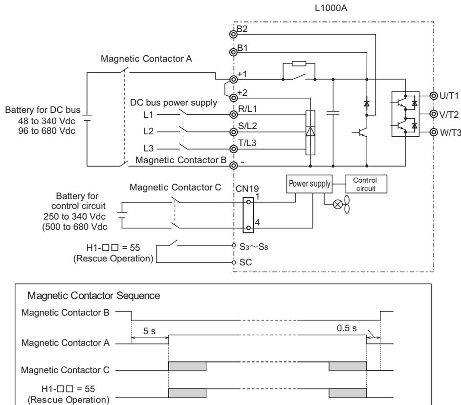
Figure 4.20 Wiring Two Batteries for DC Bus and Control Power Supply (DC Bus Battery is less than 250 V)
