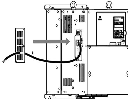
**Figure 4.32 Reattaching the CN19 Connector Cover**
