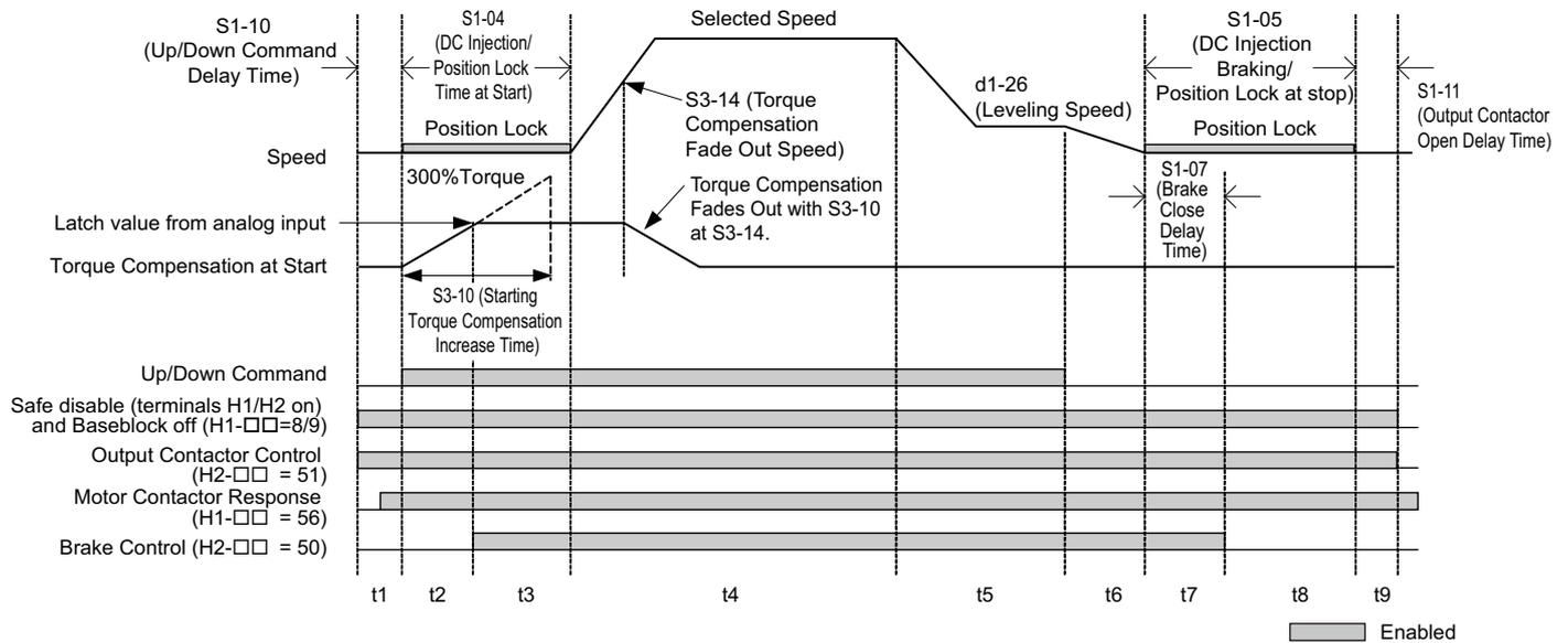
Figure 4.16 Brake Sequence Using Torque Compensation at Start
