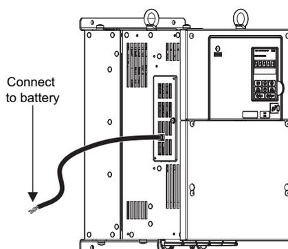
Figure 4.35 Drive and Battery CN19 Connection Complete
