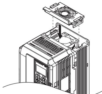
**Figure 7.6 Reattach the Fan Cover: 2A0018 to 2A0075, 4A0009 to 4A0039**
