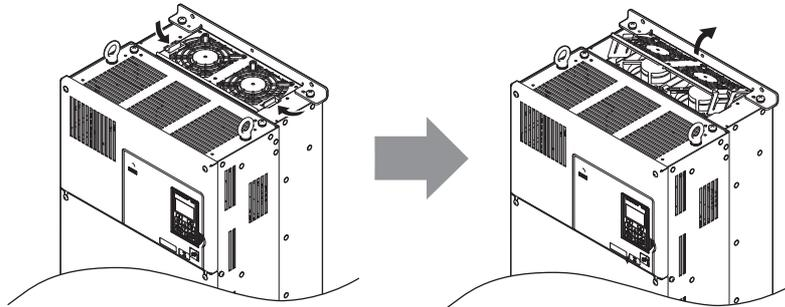
Figure 7.13 Removing the Cooling Fan Cover: 4A0075, 4A0091
