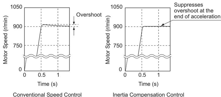
**Figure 5.41** Overshoot Suppression by Inertia Compensation
