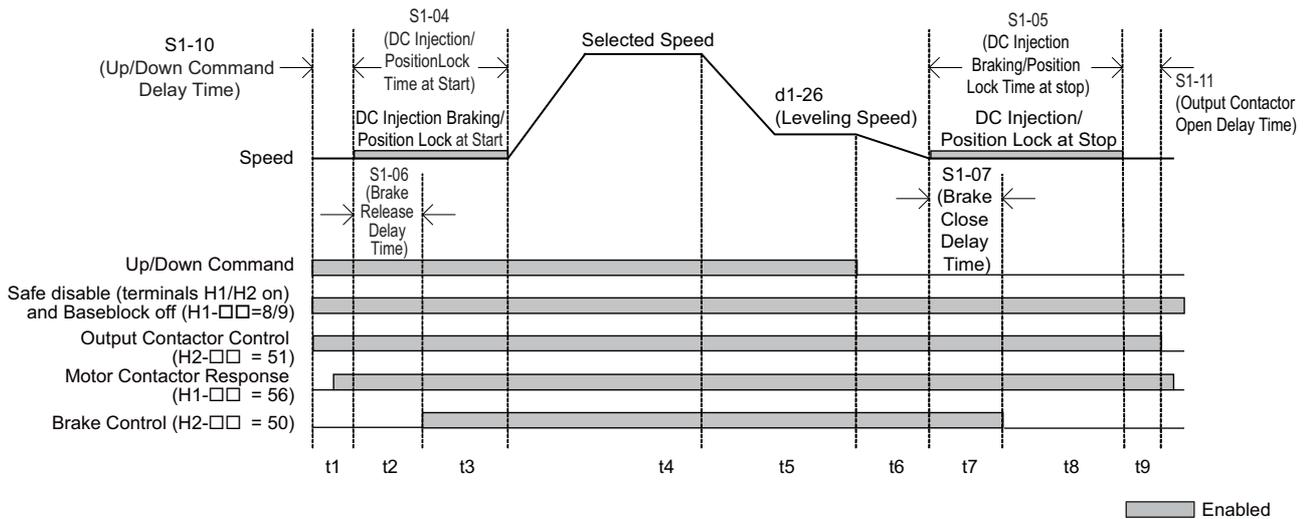
Figure 4.15 Brake Sequence without Torque Compensation at Start
