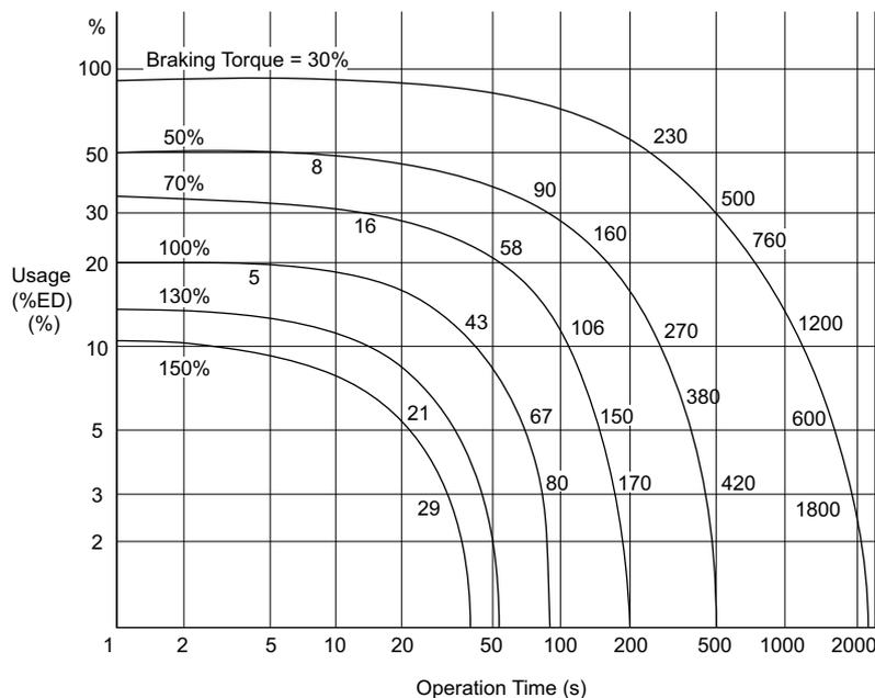
Figure 5.40 Overload Tolerance for Braking Transistor (CIMR-L□2A0018 to 2A0115, CIMR-L□4A0009 to 4A0060)
