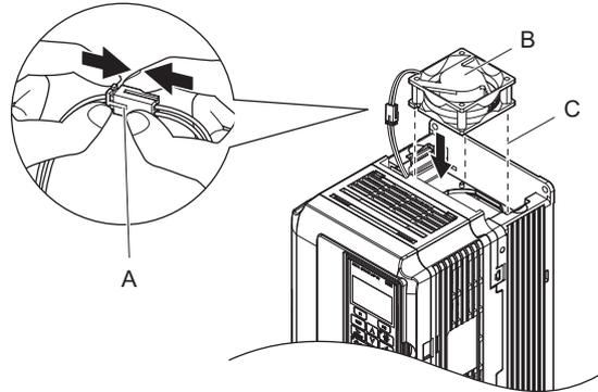
**A – Push the connectors together completely**
