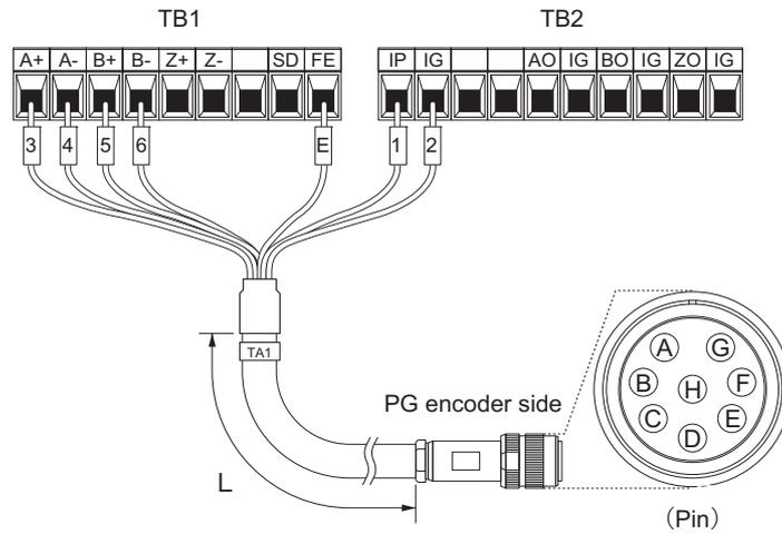
Figure 8.10 Wiring PG Encoder Cable
