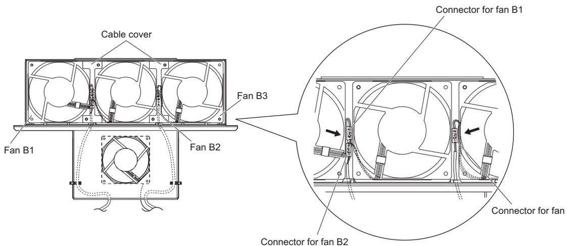
Figure 7.24 Cooling Fan Wiring: 2A0346, 2A0415, and 4A0216
