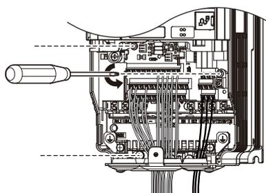
Figure 7.28 Drive Replacement: Removing the Control Terminal Board
