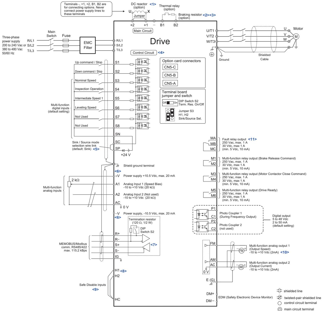
**Figure 3.1 Drive Standard Connection Diagram (example: CIMR-LC2A0033)**
