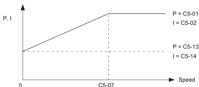
Figure 5.12 Settings at Low and High Speed during Deceleration (Leveling Speed is Selected)
