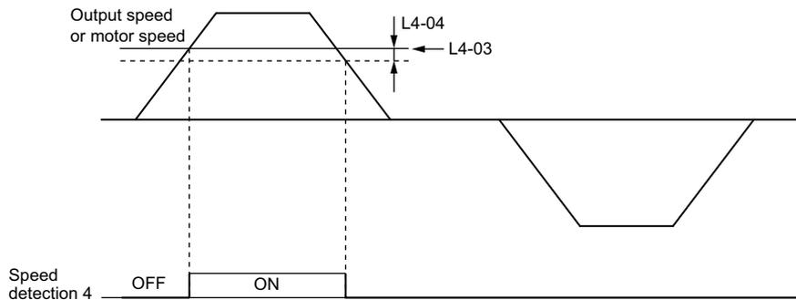
Figure 5.26 Speed Detection 4 Example with Positive L3-04 Value
