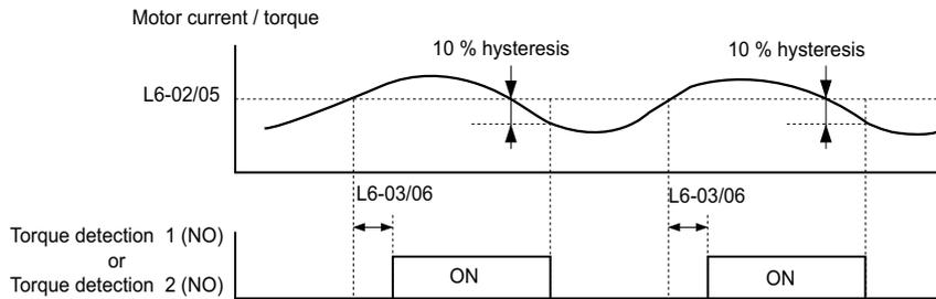
Figure 5.37 Overtorque Detection Operation
