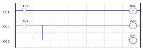
\*\* The state of auxiliary relays "M01~M3F" will be kept when the smart powers down if "M Keep" is active. "M Keep" can be set by the two ways below.
