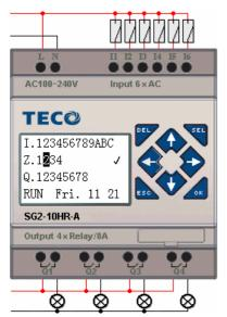
Press "←" (Z02) to disable H03 coil, and the LCD display changes to initial frame.
