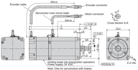
Holding brake torque = Motor rated torque
