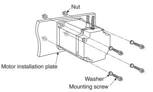
• Do not apply shock directly to the output shaft or encoder when mounting the motor, because the servomotor shaft is directly coupled to the encoder. The encoder may be damaged by the shock.
