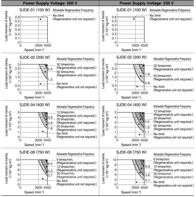
Note: An overvoltage alarm will occur if the regenerative frequency exceeds its allowable limit. This may cause a failure of the regenerative unit.
