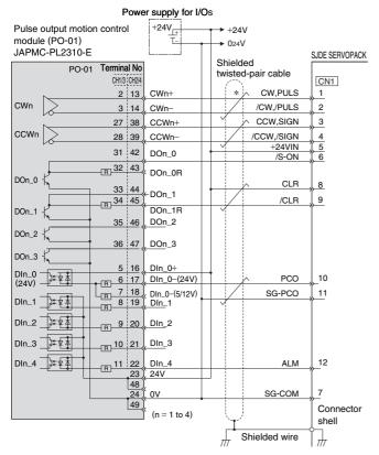
Note: Only the signals between the SJDE SERVOPACK and the pulse output motion control module (PO-01, JAPMC-PL2310-E) are shown in the diagram.
