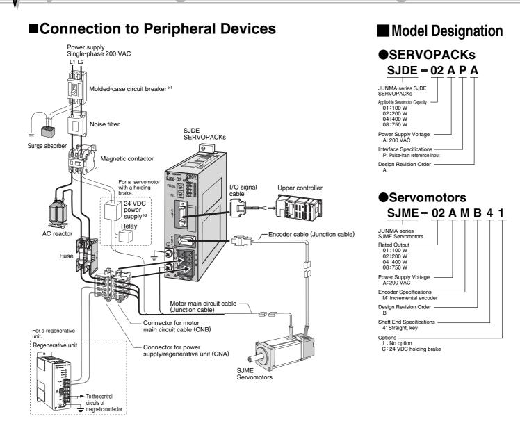
\*1 : Install a ground fault interrupter to protect against both overloads and shortcircuits, or install a ground fault interrupter for ground fault protection and a molded-case circuit breaker.
