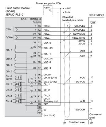
Note: Only the signals between the SJDE SERVOPACK and the pulse output module (PO-01, JEPMC-PL210) are shown in the diagram.
