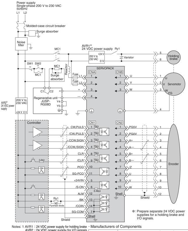
AVR2 : 24 VDC power supply for I/O signals Surge absorber Okaya Electric Industries Co., Ltd. (Spark killer): CRE-50500 SW1 : Power off switch SW2 : Power on switch Flywheel diode Toshiba Corp.: 1NH42 MC1 : Magnetic contactor Relay for holding brake Omron Corp.: MY series : Relay for holding brake Ry1 Nippon Chemi-Con Corp.: TNR7V121K Varistor
