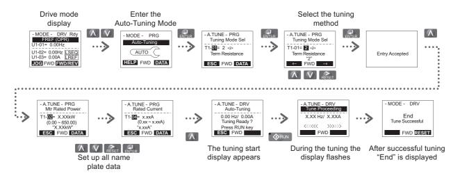
If Auto-Tuning can not be performed for some reason (no-load operation impossible etc.), then set up the maximum frequency and voltage in the E1- $\Box\Box$  parameters and enter the motor data manually into the E2- $\Box\Box$  parameters.
