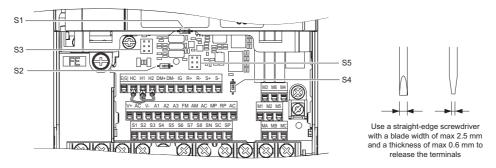
There are three DIP switches and two jumpers, S1 to S5, located on the terminal board.
