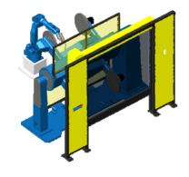
Robot cell with positioner and MOTOMAN-UP20
