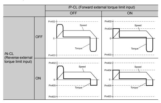
In this example, the servomotor rotation direction is Pn000.0 = 0 (CCW = forward).
