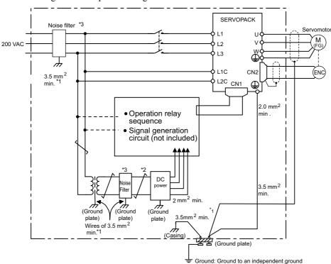
The following is an example of wiring for noise control.
