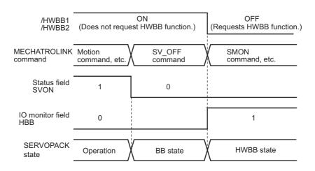
The HWBB function operates after the servomotor power is turned OFF.
