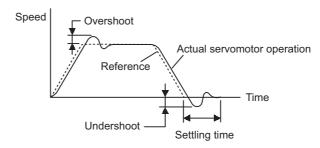
The mode switch changes the speed-control mode to PI control or P control in accordance with the setting of Pn10B.0.
