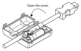
3. Remove the old battery and mount the battery (JZSP-BA01) as shown below.
