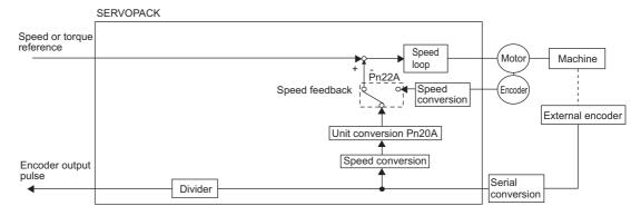
Use Pn22A.3 to select the speed feedback method during fully-closed loop control: Normally, set Pn22A.3 to 0 (Uses motor encoder speed.). Set Pn22A.3 to 1 (Uses external encoder speed.) when connecting a direct drive motor and high-resolution external encoder.
