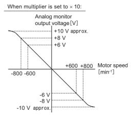
Note: Linear effective range: within ± 8V Encoder resolution: 16-bit
