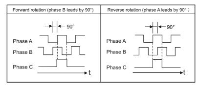
Note: The pulse width of the (Phase C origin pulse) changes according to the setting of the Pn212 and becomes the same as that for phase A.
