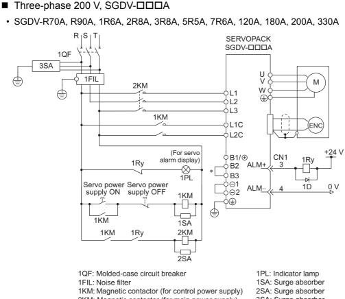
2KM: Magnetic contactor (for main power supply) 1Ry: Relay
