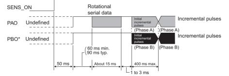
\* In case of reverse rotation mode (Pn000.0 = 1), the output polarity for PBO signal inverts.
