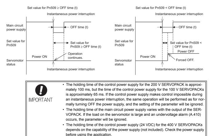
If the uninterruptible power supplies are used for the control power supply and main circuit power supply, the SERVOPACK can withstand an instantaneous power interruption period in excess of 1000 ms.
