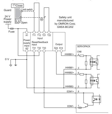
When a guard opens, both of signals, the /HWBB1 and the /HWBB2, turn OFF, and the EDM1 signal is ON. Since the feedback is ON when the guard closes, the safety unit is reset, and the /HWBB1 and the /HWBB2 signals turn ON, and the operation becomes possible.
