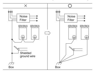
If a noise filter is located inside a control panel, connect the noise filter ground wire and the ground wires from other devices inside the control panel to the ground plate for the control panel first, then ground these wires.
