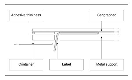
The label in the figure is free and does not cause tension on the keyboard.
