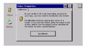
From the control panel click on the stylus icon and, subsequently, the following screens are displayed on the recalibrate key. Touch the screen near the crosses that appear on the screen.
