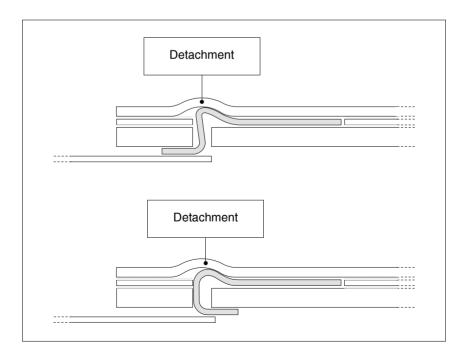
The labels in the figure generate forces, which through time, may cause detachment of the keyboard.
