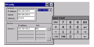
By clicking on the "IP Config" icon, the mask displaying the IP Address of the terminal and IP Address (or IP Addresses) of the devices connected via Ethernet will appear.
