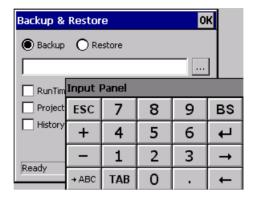
A backup copy of the components chosen through ticking can be made from here: Runtime, Project, History.
