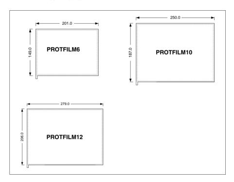
It is a transparent protection film to apply onto the front of the touch screen terminal to protect it from wear by external agents (see chap. 20, "Resistance to chemical substances" page 259).
