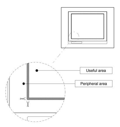
The peripheral area is about 2 mm per side and is outside of the sensitive area.
