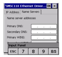
f necessary, the parameters relating to the relative DNS or AL WINS must be entered
