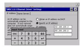
Obtain an IP address via DHCP: by selecting this option, an IP address is automatically obtained (ensure that the DHCP server is enabled on the network)
