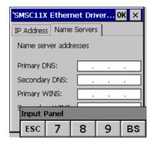
If necessary, the parameters relating to the relative DNS or AL WINS must be entered
