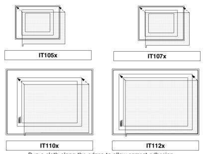
• Run a cloth along the edges to allow correct adhesion
