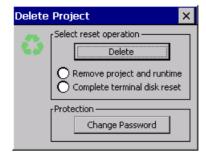
"Reset" is an application of the terminal control panel which allows to cancel all that been transferred onto the Hard Disk. Selecting the "Enable" option, the "FTP" folder sharing service in the "Hard Disk" directory is enabled.
