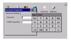
The Password option allows assigning a password to the terminal.
