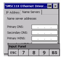
If necessary, the parameters relating to the relative DNS or AL WINS must be entered
