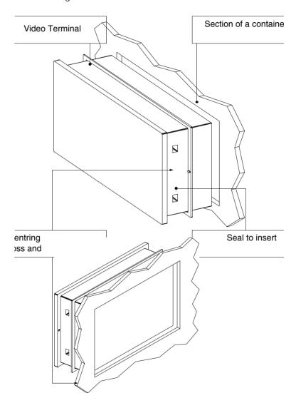
After having prepared the container that will house the terminal: Insert the seal in the terminal respecting the direction of insertion indicated by the centring bosses
