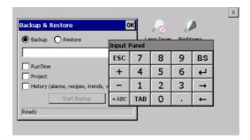
A backup copy of the components chosen through ticking can be made from here: Runtime, Project, History.
