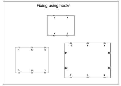
Perform the initial tightening of the fixings with a moderate force in a way to allow uniform adhesion in all points, once all fixings have been tightened repeat the definitive tightening sequence.
