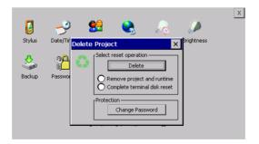
"Reset" is an application of the terminal control panel which allows to cancel all that been transferred onto the Hard Disk. Selecting the "Enable" option, the "FTP" folder sharing service in the "Hard Disk" directory is enabled.
