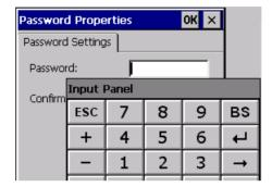
The Password option allows assigning a password to the terminal.
