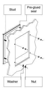
After having prepared the container that will house the terminal: Insert the terminal into the slot Keep the terminal against the wall Insert the washer follwed by the nut into the studs
