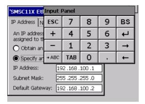
Obtain an IP address via DHCP: by selecting this option, an IP address is automatically obtained (ensure that the DHCP server is enabled on the network)
