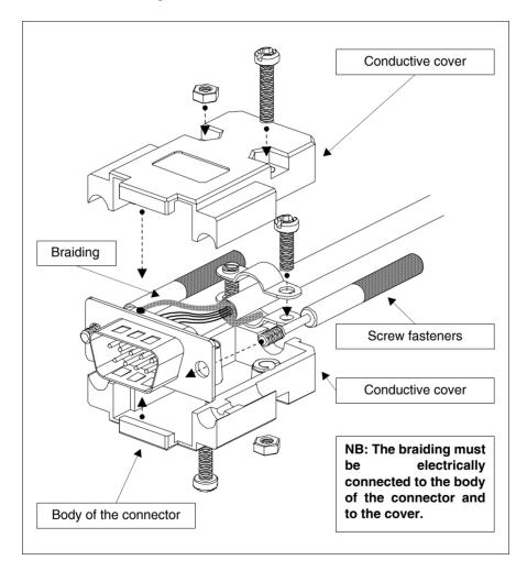
The interface cable shield must be electrically connected to the case and to the body of the connector itself from both sides of the cable.
