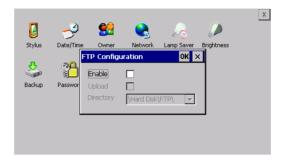
The "FTP" acronym means "Files Transfer Protocol". It gives the user the possibility to enable and disable the "FTP Server" service of the panel from any other device (PC,XS,IT,YT) connected to the network.
