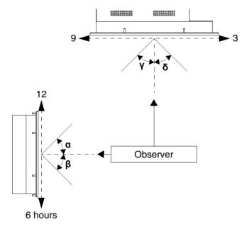
The figure shown above shows the direction of the angles depending on the observation point. The table states the value of the display angles depending on the type of
