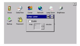
By enabling the Lamp Saver, the lamp switches off after a time set in the Wait box.
