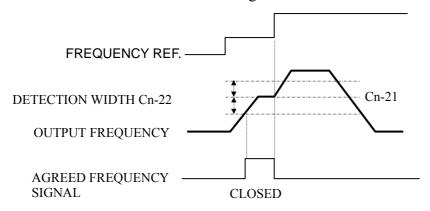
(Cn-21 - Cn-22) Output frequency (Cn-21 + Cn-22)
