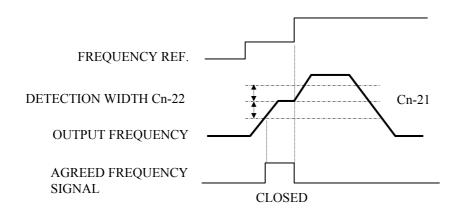
(Cn-21 - Cn-22) Output frequency (Cn-21 + Cn-22)
