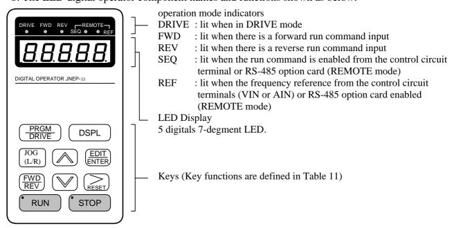
Fig 9-b LED Digital operator component names and functions
