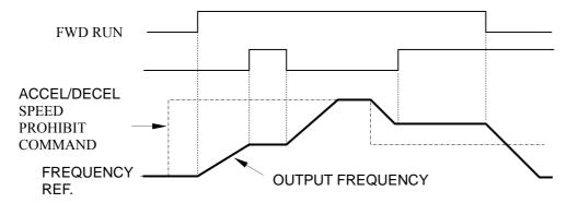
Note: If the run command is input again after the stop command is input while the accel/decel prohibit command is input, the holding output frequency is stored unless the accel/decel prohibit command is released. Therefore, operation is performed at the stored output frequency. Also when the power supply is turned OFF in the accel/decel prohibit command input status, the holding output frequency is still stored.
