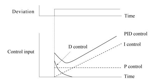
Fig. 14 PID Control Operations
