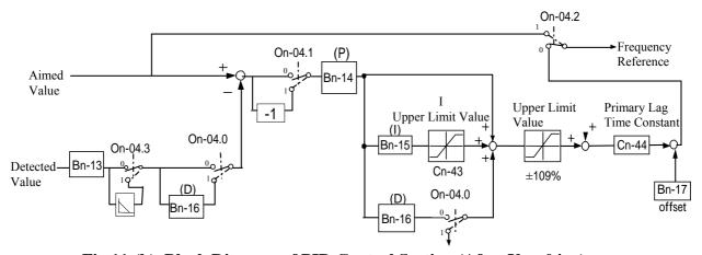
Fig 11-(b) Block Diagram of PID Control Section (After Ver. 04xx)
