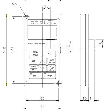
Fig. 6 LCD Digital Operator Dimension
