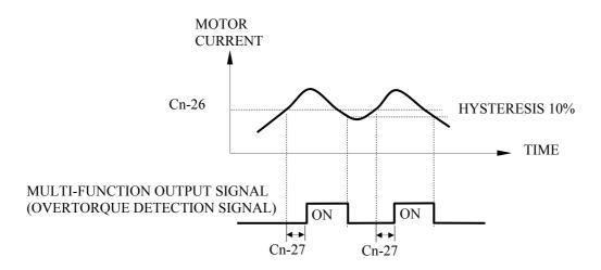
Setting either Sn-20 to 22 to "OB" enables signal to be output at overtorque detection.
