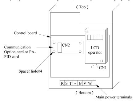
Fig. 8 Option card Installation
