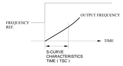
Note: S-curve characteristics time refers to the time from acceleration rate 0 to the time when a normal acceleration rate determined by a specified acceleration time is obtained.
