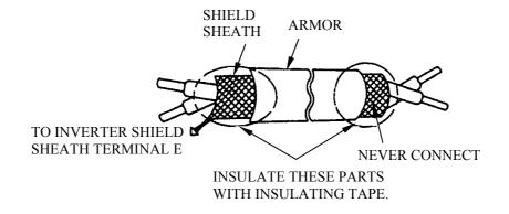
Fig. 4 Shielded Wire Termination
