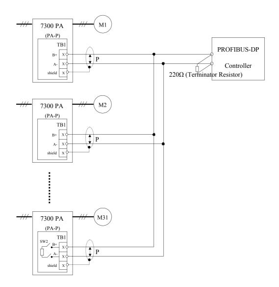
Fig. 16 Wiring for PROFIBUS protocol communication
