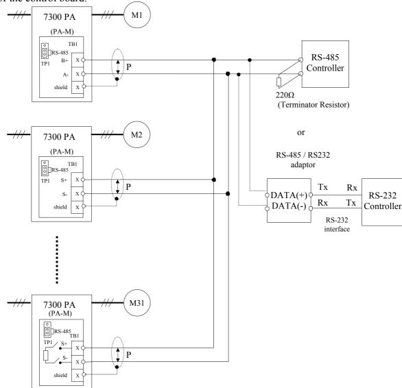
Fig. 15 Wiring for PA-M MODBUS Protocol communication
