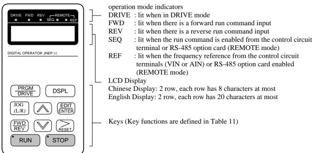
Fig 9-a LCD Digital operator component names and functions
