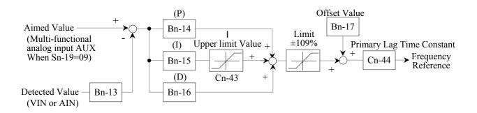
Fig 11-(a) Block Diagram of PID Control Section
