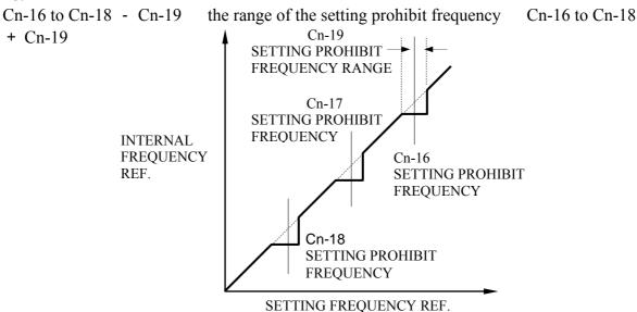
Note: Constant-speed operation is prohibited in the setting prohibit frequency range. Output frequency does not jump during acceleration or deceleration, which is performed smoothly.
