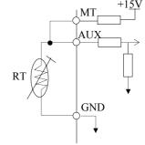
• The motor overheat (OH3) alarm can be reset when  $R_T = 550\Omega$ .
