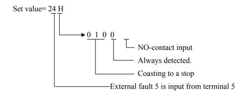
The inverter operates differently as described below when Experiencing major faults or minor faults. The digits in the error display Ext. Fault 5 to 8 (EF5 to EF8) indicate the terminal numbers in which external faults 5 to 8 are set.
