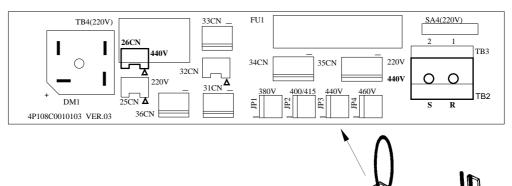
Fig. 5 Voltage Selecting Connector
