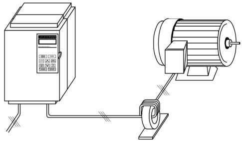
Note: All the line wire of U/T1, V/T2, W/T3 phase must pass through the same zero-phase core in the same winding sense.
