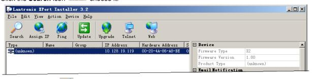
5. Click the **Ping** icon Ping button. The results display in the Status area, make sure the unit is properly attached to the network and that the IP address assigned is valid for the particular network segment you are working with. Click the **Close** button
