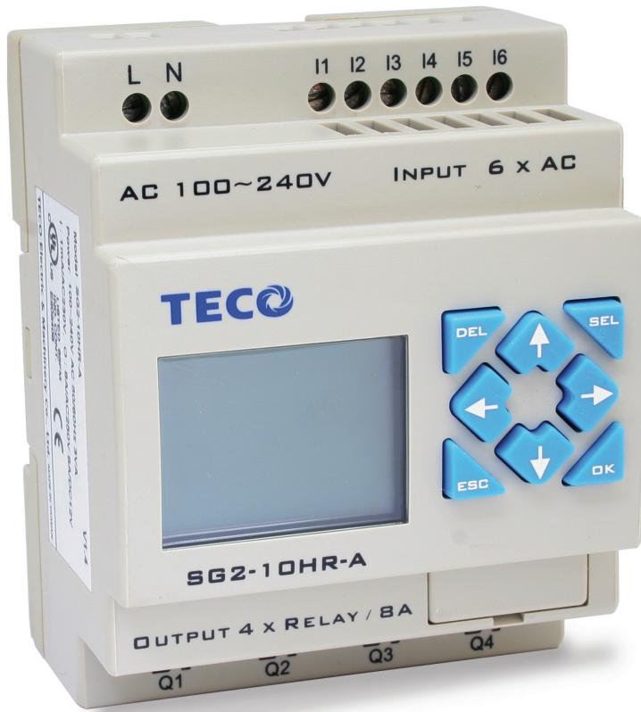
**SG2 Programmable Logic Relay**
