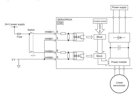
Note: For safety function signal connections, the input signal is the 0V common and the output signal is the source output. This is opposite to other signals described in this manual. To avoid confusion, the ON and OFF status of signals for safety functions are defined as follows:
