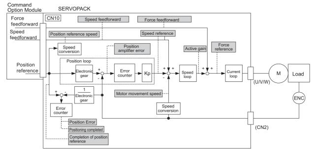
The following signals can be monitored by selecting functions of parameters Pn006 and Pn007. Pn006 is used for analog monitor 1 and Pn007 is used for analog monitor 2.
