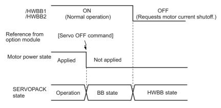
The HWBB function operates during the linear servomotor operation.
