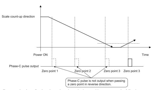
To output the phase-C pulse when a detection point is passed in reverse, set the following parameter to 1.
