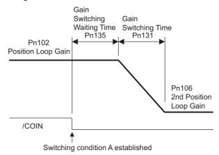
Note: Automatic gain switching is available in the PI and I-P controls. (Pn10B)
