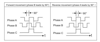
Note: The pulse width of the phase C (origin pulse) changes according to the setting of the Pn281 and becomes the same as that for phase A.
