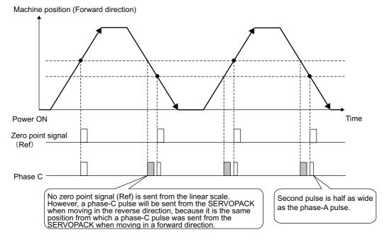
• When Passing 1st Zero Point Signal (Ref) in Reverse Direction and Returning after Power ON
