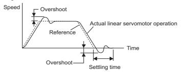
To enable the mode switch, set Pn10B.0 to 0 to 3. The mode switch changes the speed-control mode to PI (proportional/integral) control or P (proportional) control.
