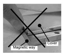
When removing the dummy plate for reducing magnetic force used for the SGLFW magnetic way, pay attention to the magnetic attraction of the magnetic way. Do not place the removed plate close to the magnetic way.
