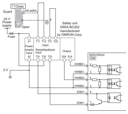
When a guard opens, both of signals, the /HWBB1 and the /HWBB2, turn OFF, and the EDM1 signal is ON. Since the feedback circuit is ON when the guard closes, the safety unit is reset, and the /HWBB1 and the /HWBB2 signals turn ON, and the operation becomes possible.
