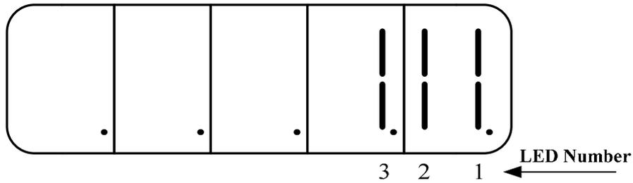
When output terminal signal has a low logic level (**close** loop with **IG24**), the corresponding LED will be on.
