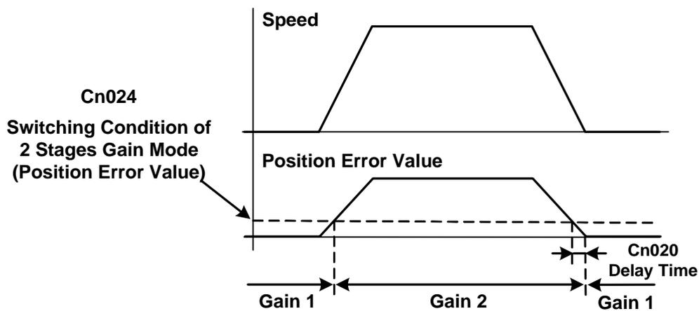
**(5) Automatic gain 1&2 switch condition by G-SEL input contact.**
