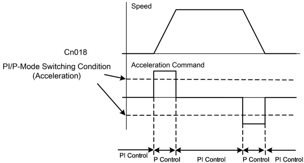
(4) **PI to P mode switch over by comparing *Position Error value*.**
