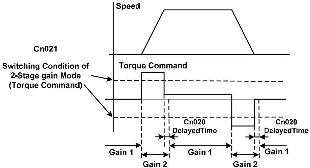
**(2) Automatic gain 1&2 switch condition (by Speed command).**
