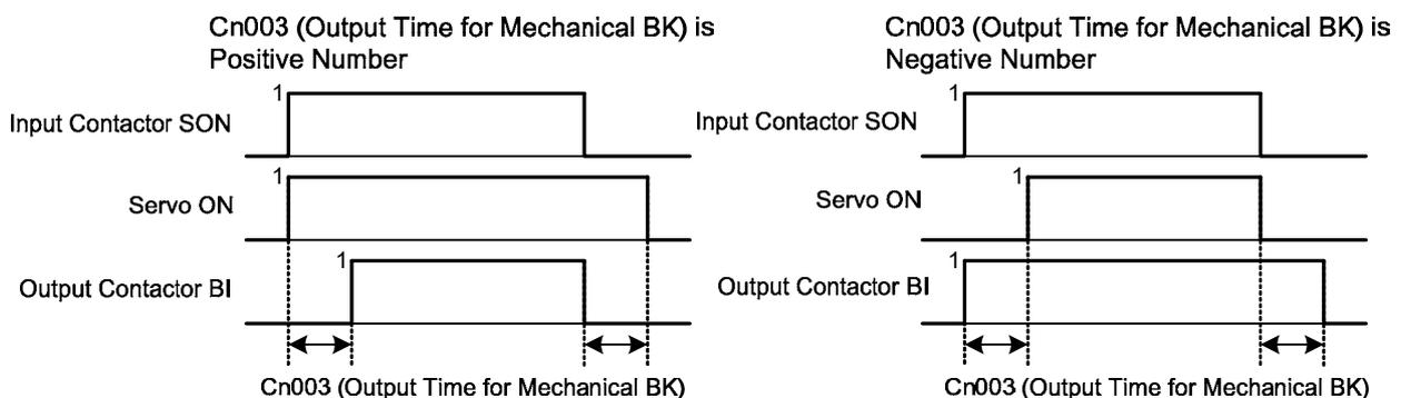
Note: Input contacts status of above time sequence diagram "1" (ON) and "0" (OFF).
