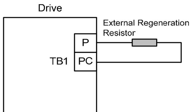
When installing Regeneration Resistors care must be taken as the resistor absorbs the regeneration power, and it is possible to generate the high temperatures above 100°C.
