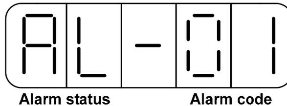
For Alarm List refer to the section 8-2. In the example above AL-01 indicates (Under Voltage)
