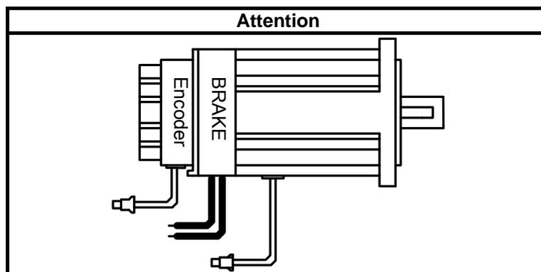
2. Vertical Install: If the motor shaft is side-up installed and mounted to a gear box, please pay attention to and avoid the oil leakage from the gear box.
