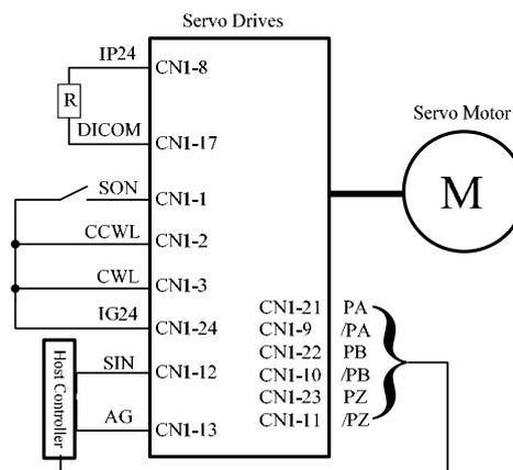
**5. Confirm the rotation number and encoder output of Servo Motor.**
