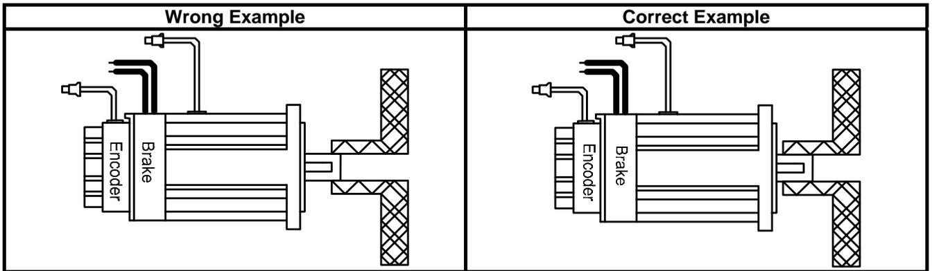
5. Please do not beat the motor when installing or taking it apart. Otherwise the shaft and the encoder of backside will be damaged.
