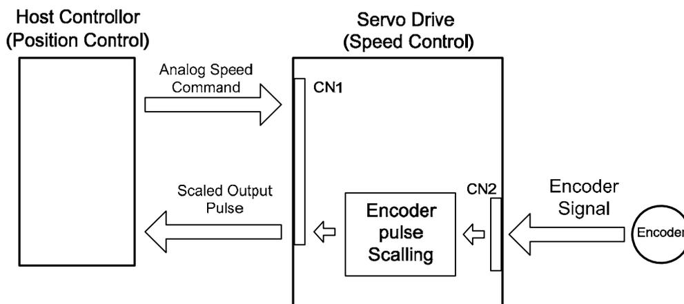
Set the required encoder Pulse Per Revolution (PPR) in parameter Cn005.
