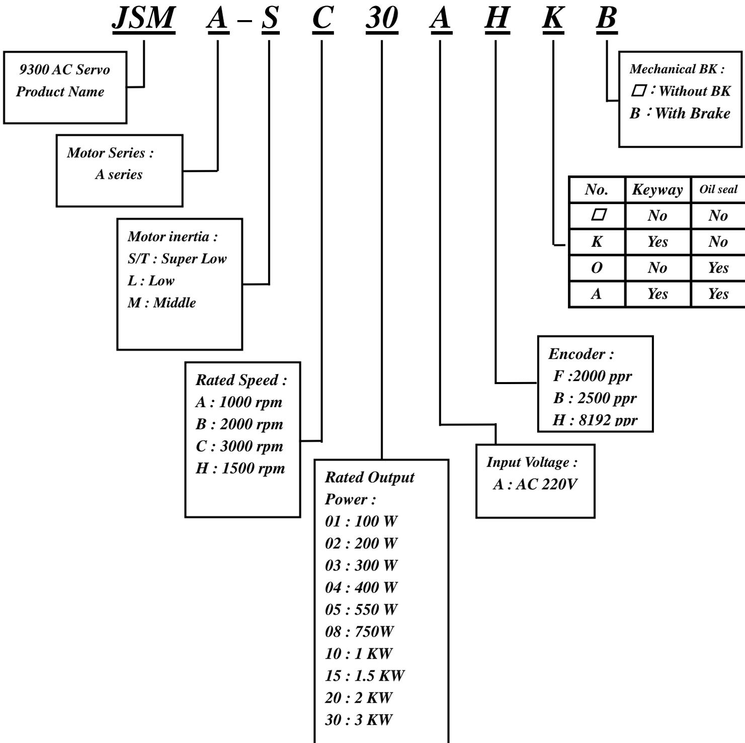
※ Standard Specifications for Low Inertia and Super Low Inertia
