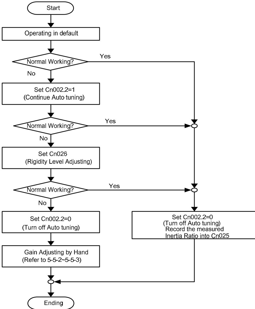
Note: After Auto tuning is complete Set 0 in Cn002.2, otherwise it will not record the present measured Load Inertia Ratio.
