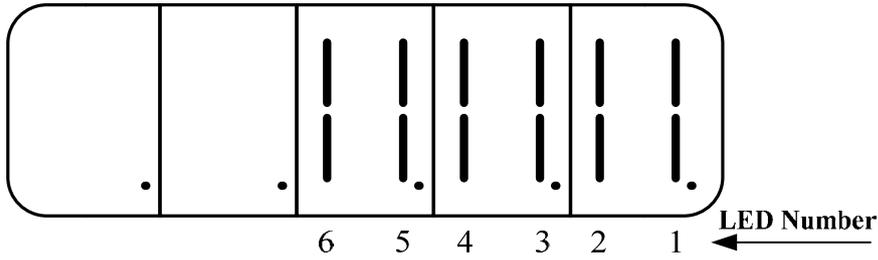
When Input terminal signal has a low logic level (close loop with **IG24**), the corresponding LED will be on.
