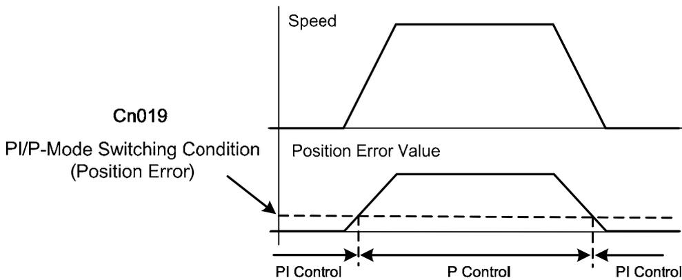
(5) **PI to P mode switch over by PCNT input contact.**
