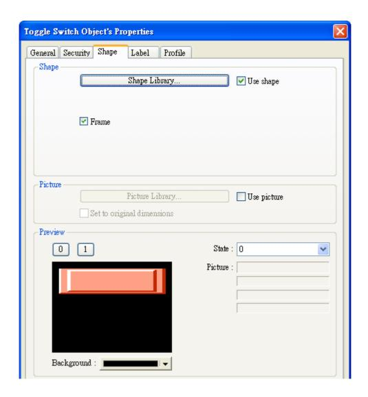
And then double click this object to call up Toggle Switch Object's Properties / Profile tab.
