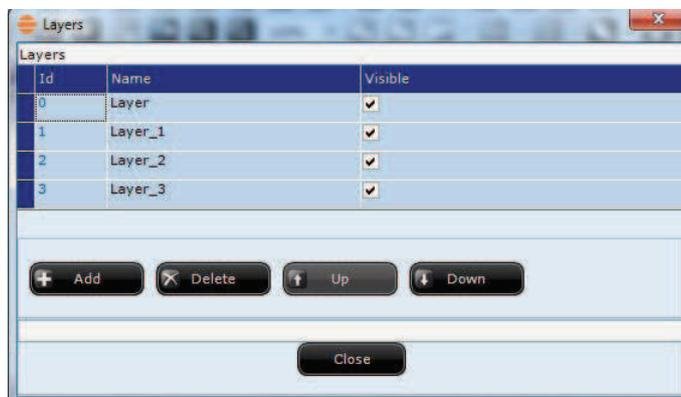
This function allows a **division of the project pages** being edited **into levels**, so that it is easier to create them and, more importantly, **make any subsequent changes**. This way it is possible to **position the various elements of the page on different levels**, so that it is easier to move them, delete them, make them interact and modify them.
