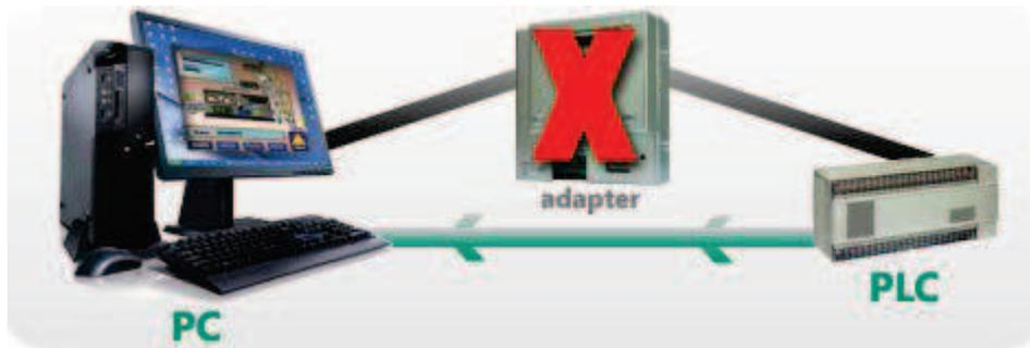
**Polymath Machine Edition**, the **ESA's runtime** tool to execute **Polymath projects** on **PCs**, can now **directly manage serial** communication of the following protocols:
