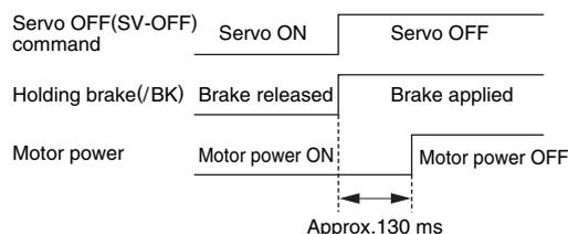
② When the servo is OFF while the servomotor is running.
