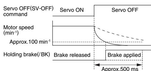
/BK signal turns ON when either of the following is satisfied while the servomotor is rotating.
