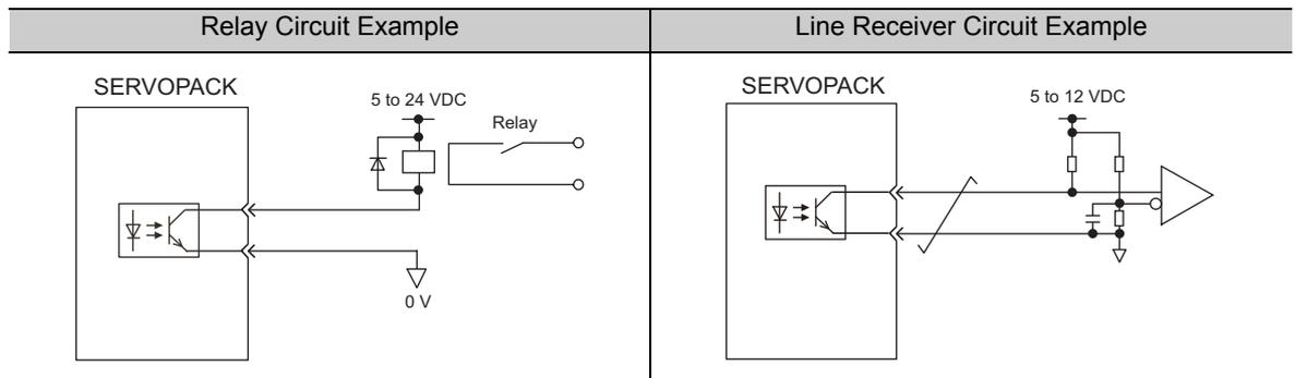
Note: The maximum allowable voltage and current capacities for photocoupler output circuits are as follows.
