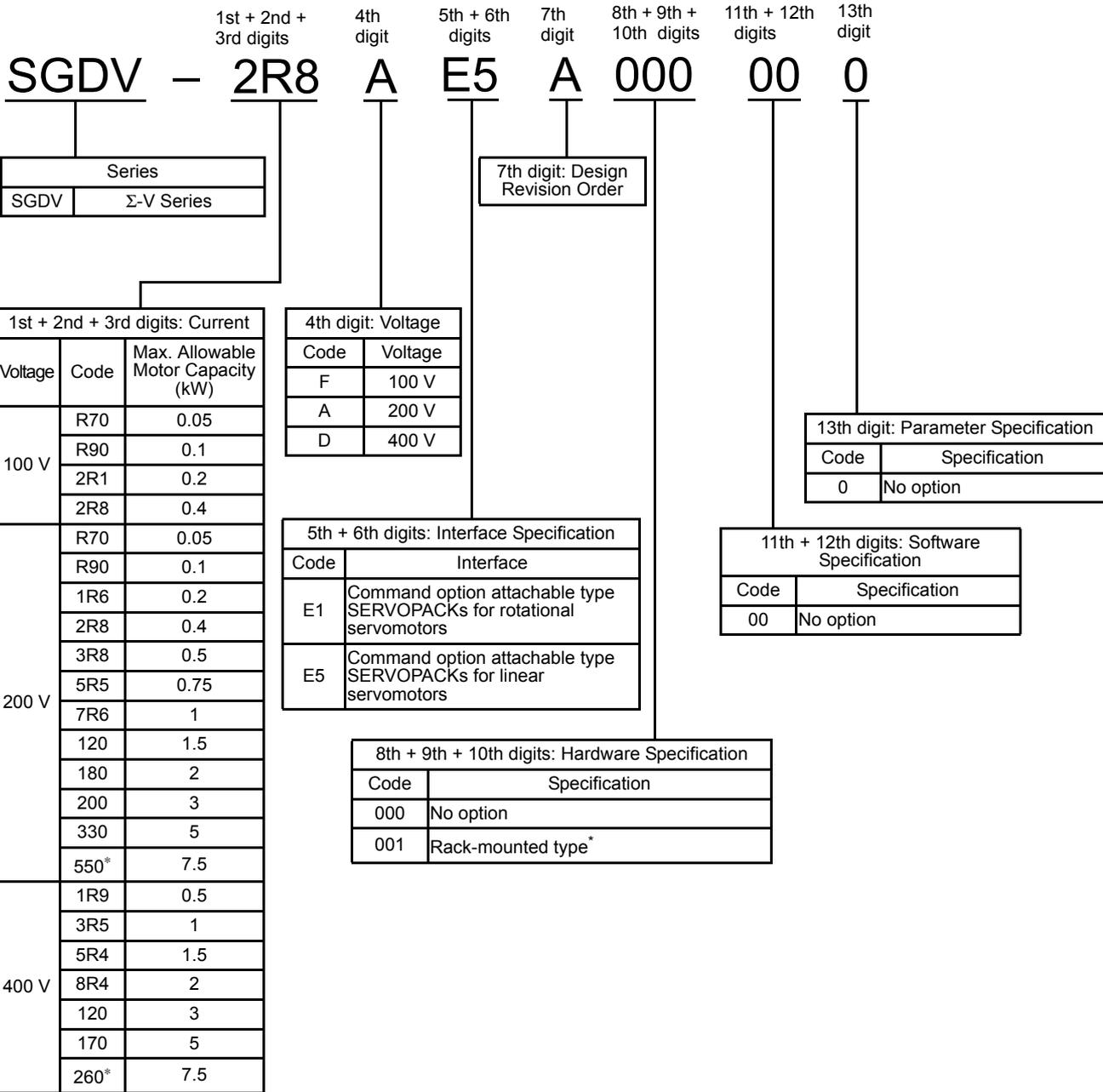
\* The SGDV-550A and -260D have air ducts for ventilation.
