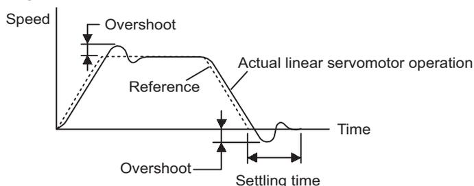
To enable the mode switch, set Pn10B.0 to 0 to 3. The mode switch changes the speed-control mode to PI (proportional/integral) control or P (proportional) control.
