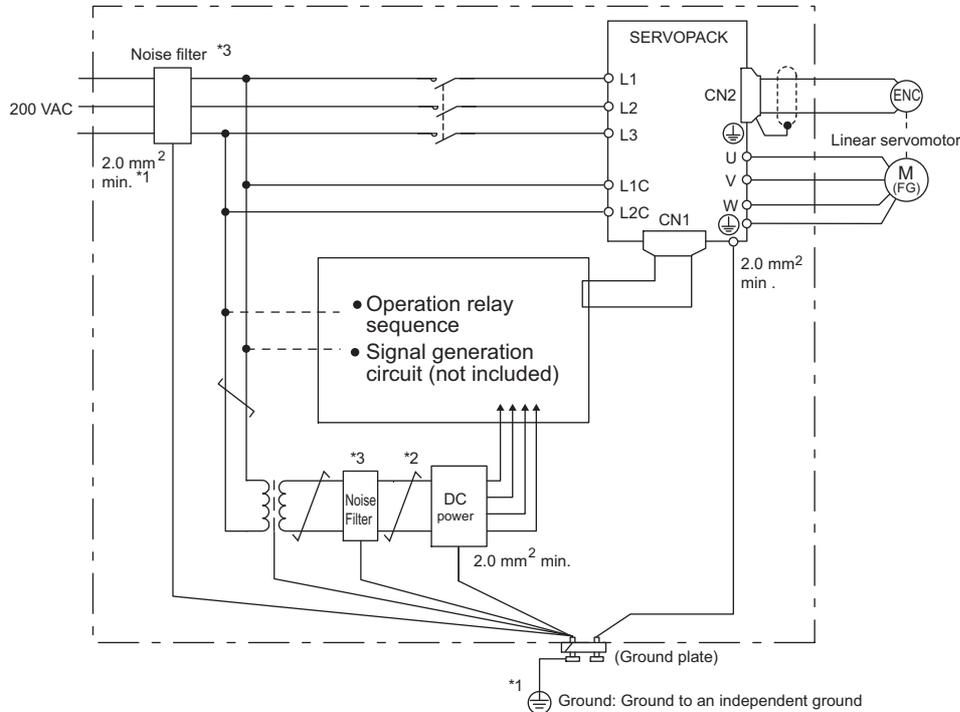
\*1. For ground wires connected to the ground plate, use a thick wire with a thickness of at least 2.0 mm<sup>2</sup> (preferably, plain stitch cooper wire).
