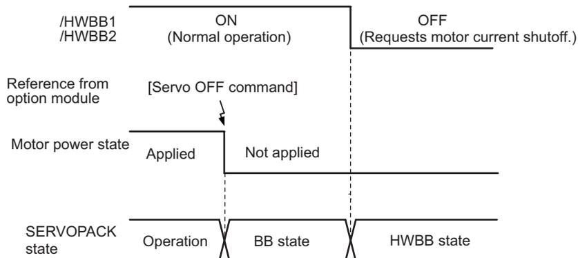
The HWBB function operates during the linear servomotor operation.
