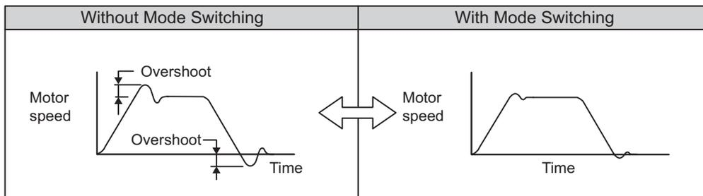
■ Using the Speed Reference Level to Switch Modes
