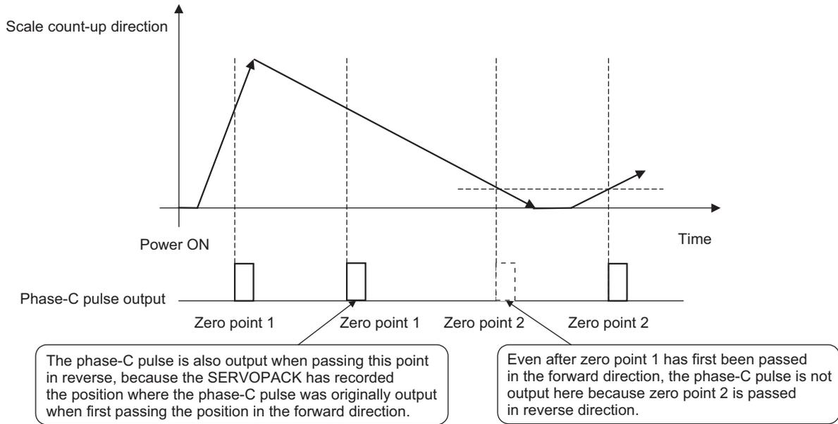
■ When Using a Linear Scale with Multiple Zero Points and Passing 1st Zero Point in Reverse Direction and Returning after Power ON
