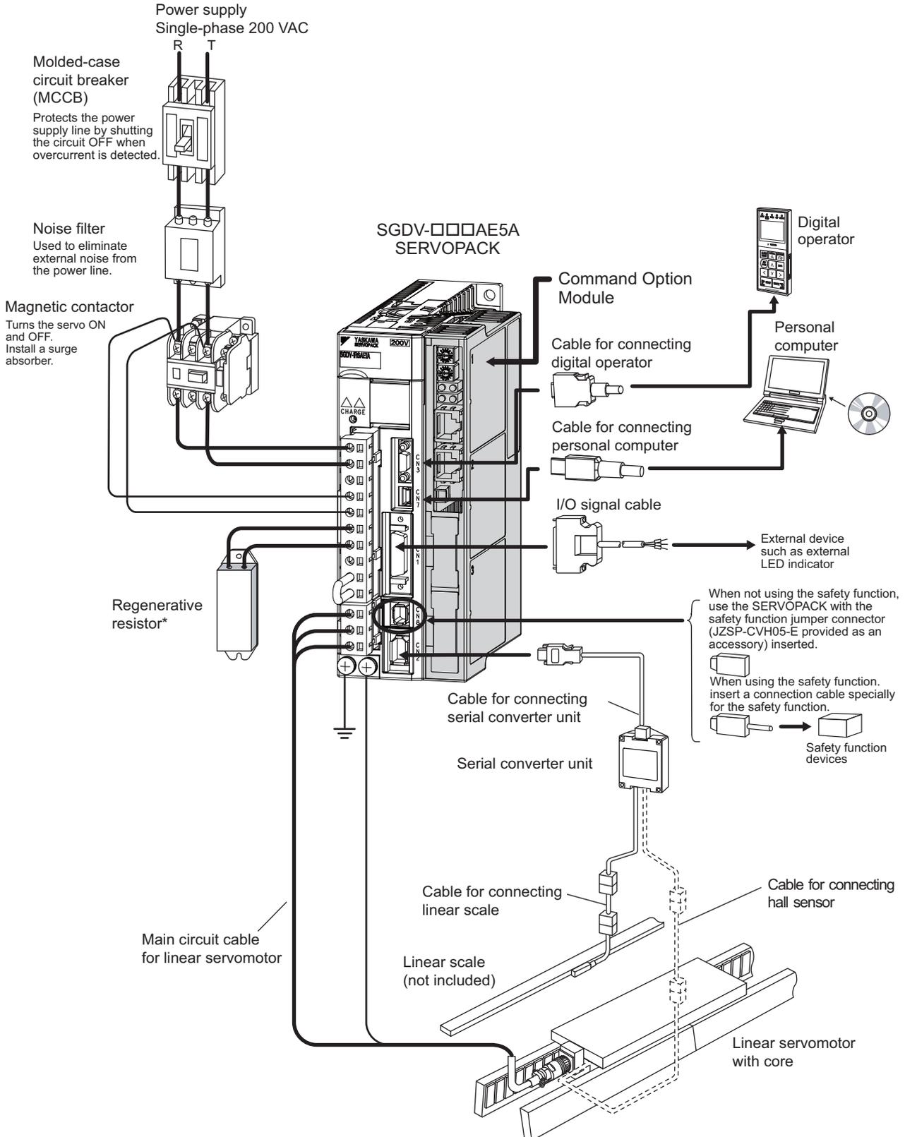
\* Before connecting an external regenerative resistor to the SERVOPACK, refer to 3.7 *Regenerative Resistors Connections*.
