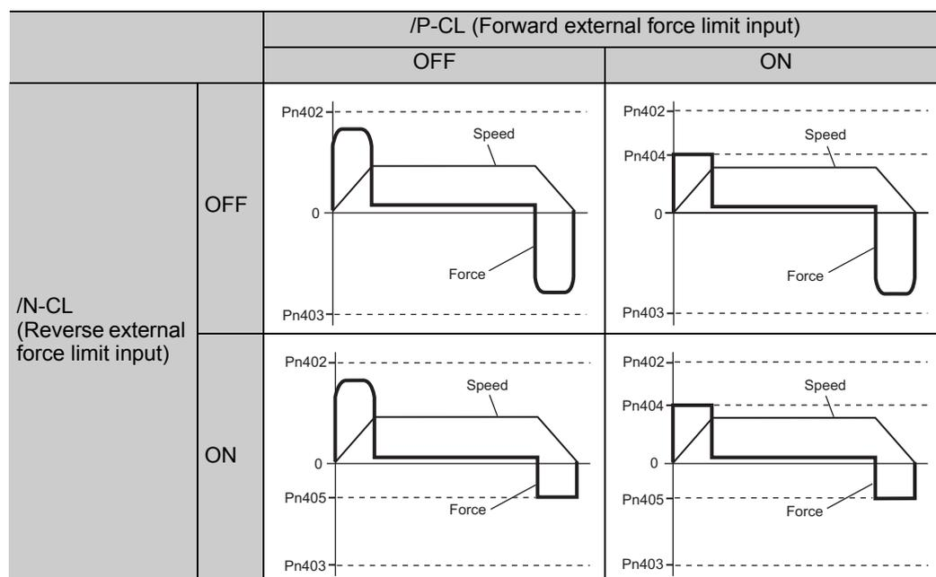
Note: The waveform reverses in case of analog monitor (CN5) output.
