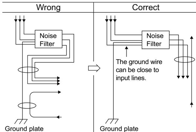
Connect the noise filter ground wire directly to the ground plate.
