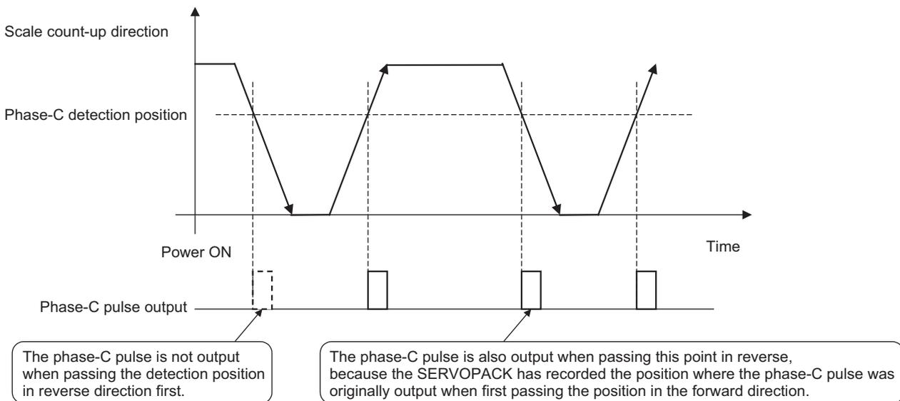
■ When Using a Linear Scale with Multiple Zero Points and Passing 1st Zero Point in Forward Direction and Returning after Power ON
