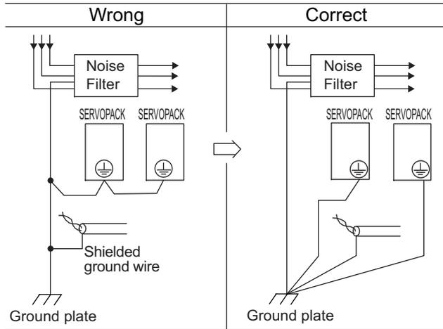
If a noise filter is located inside a control panel, connect the noise filter ground wire and the ground wires from other devices inside the control panel to the ground plate for the control panel first, then ground these wires.
