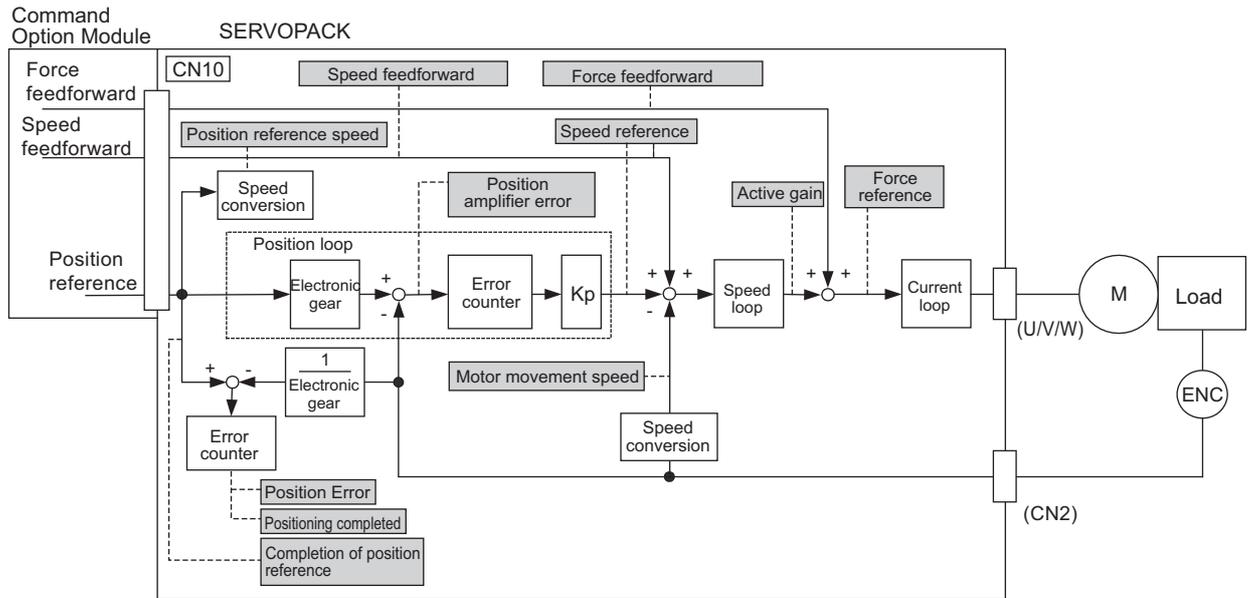
The following signals can be monitored by selecting functions of parameters Pn006 and Pn007. Pn006 is used for analog monitor 1 and Pn007 is used for analog monitor 2.
