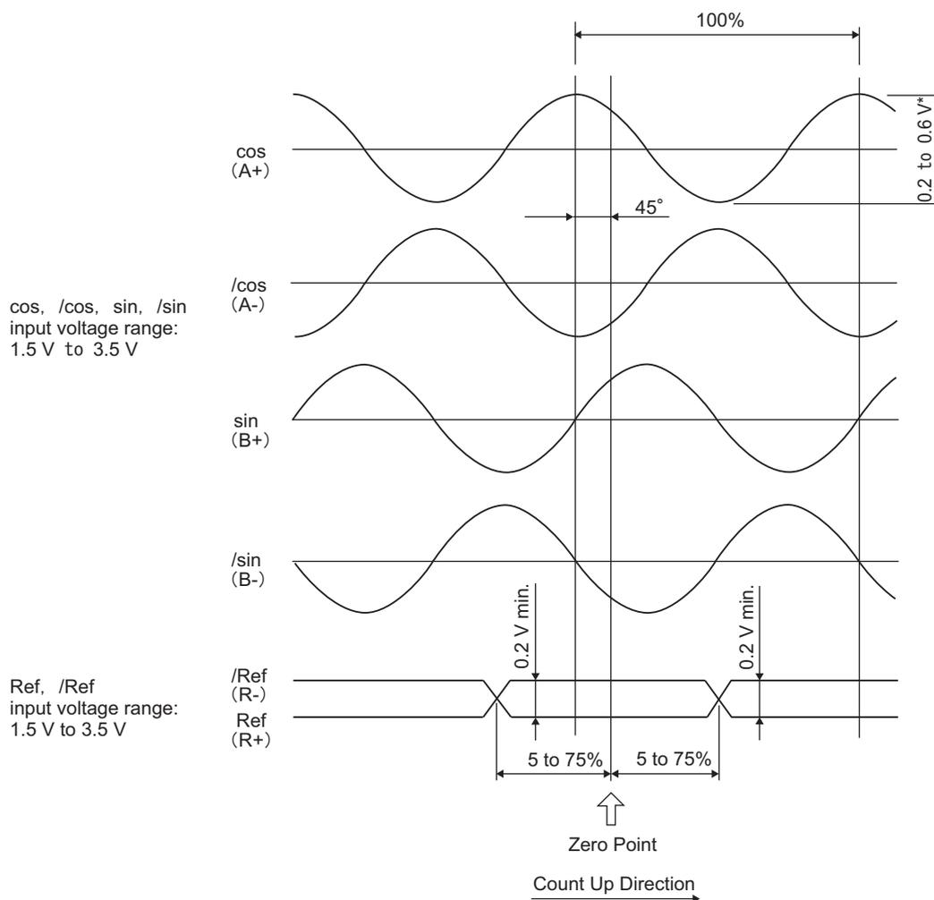
\* If the analog signal amplitude declines to about 0.35 V because of differential amplitude, the serial converter unit outputs an alarm.
