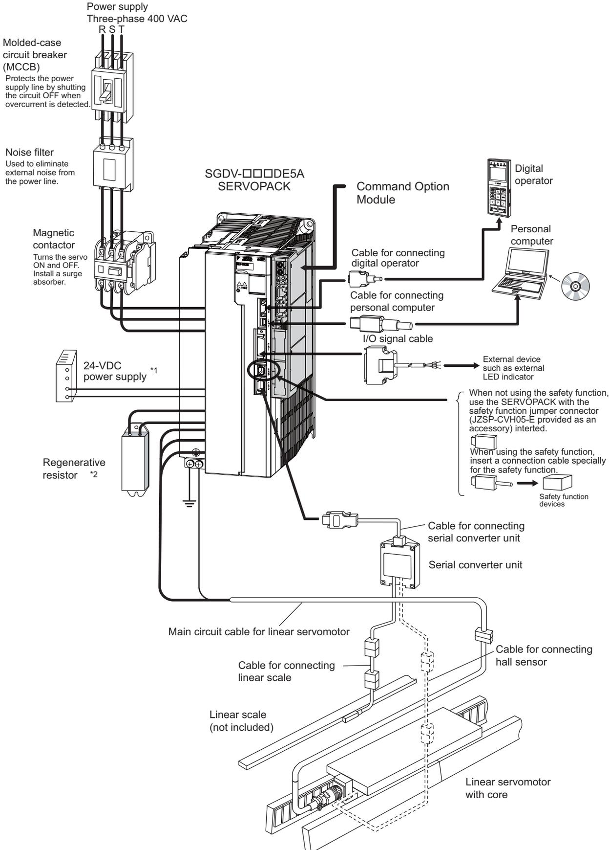
\*1. Use a 24-VDC power supply with double insulation or reinforced insulation. (The power supply is not included)
