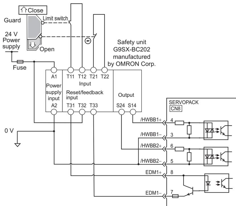
When a guard opens, both of signals, the /HWBB1 and the /HWBB2, turn OFF, and the EDM1 signal is ON. Since the feedback circuit is ON when the guard closes, the safety unit is reset, and the /HWBB1 and the /HWBB2 signals turn ON, and the operation becomes possible.
