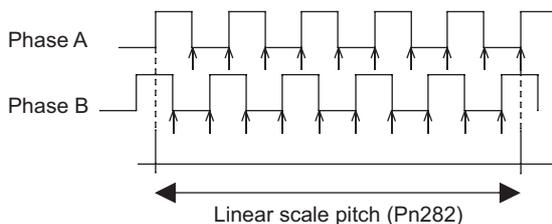
Note: When the linear scale is directly connected to the SERVOPACK and a serial converter unit is not used, Pn282 is not valid. On the Un084 and Un085 monitors, check the linear scale pitch.
