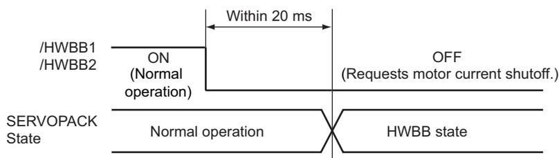
Note: The OFF status is not recognized when the /HWBB1 and /HWBB2 signals are OFF for 0.5 ms or shorter.
