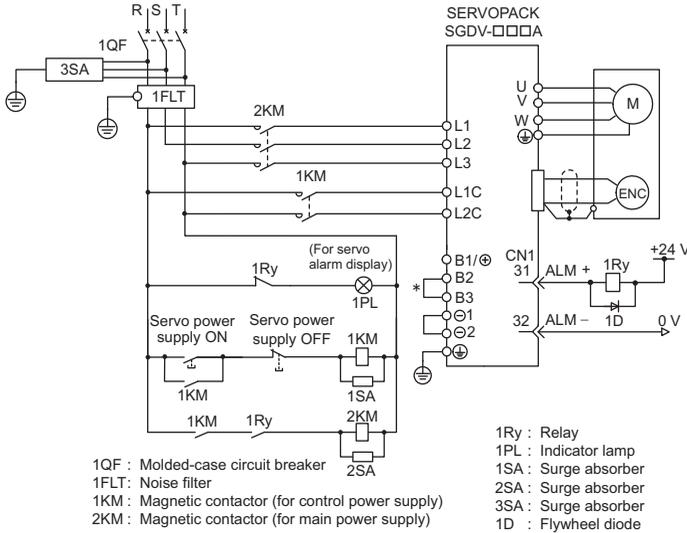
\* For SGD□-R70A, R90A, 1R6A, and 2R8A SERVOPACKS, the short-circuit between B2 and B3 is not required. Do not short the connection between B2 and B3.
