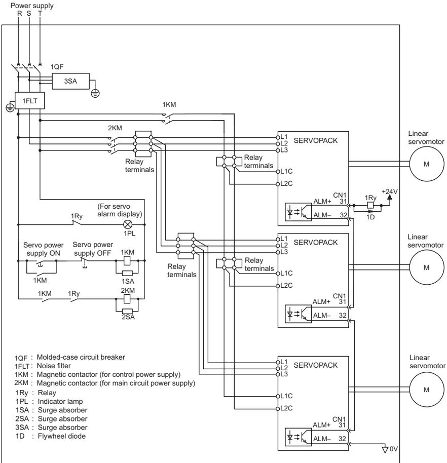
Note: For M-II model, M-III model, and command option attachable type SERVOPACKs, the pin number of ALM+ terminal is CN1-3, and that of ALM- terminal is CN1-4.
