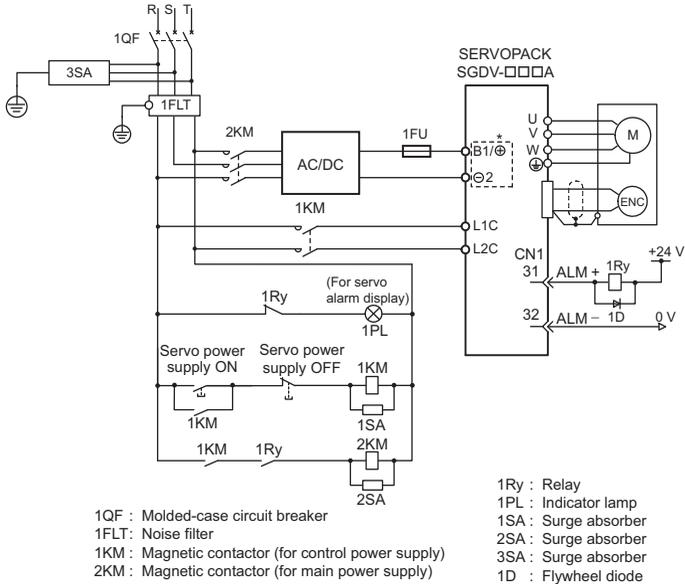
Note: For M-II model, M-III model, and command option attachable type SERVOPACKS, the pin number of ALM+ terminal is CN1-3, and that of ALM- terminal is CN1-4.
