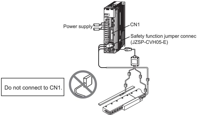
Make sure that the following cables are correctly connected.
