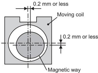
2. Take the product out of the package with the moving coil and the magnetic way being combined (same as the state when the product is delivered).
