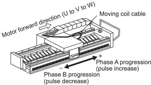
Note: When the direction of the linear servomotor and the direction in which the linear scale counts pulses are reversed because of wiring or other factors, set the parameter Pn080.1=1 (Sets phase B lead as phase sequence of U, V, W).
