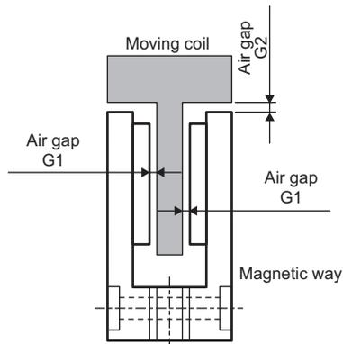
2. Move the moving coil back and forth several times over the magnetic way from end to end, making sure that the moving coil and magnetic way are not touching each other and that no foreign objects such as magnetic particles are present.
