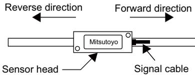
When installed as shown in the diagram on the left, operation is performed in the forward direction when the sensor head is moved to the left.
