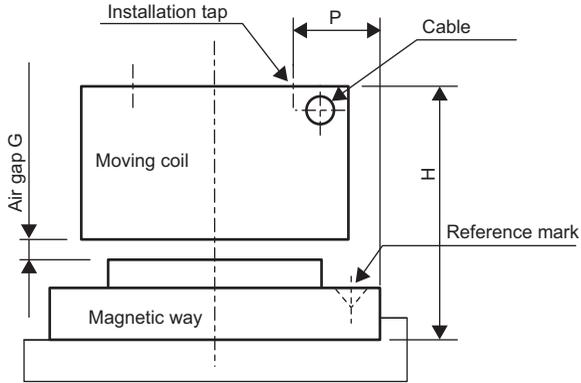
Linear servomotor side view
