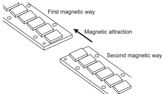
Note: To ensure your safety, install the moving coil before installing the second and subsequent magnetic ways. For details, refer to (2) *Moving Coil Installation*.
