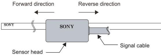
When installed as shown in the diagram on the left, operation is performed in the forward direction when the sensor head is moved to the left.
