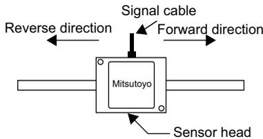
When installed as shown in the diagram on the left, operation is performed in the forward direction when the sensor head is moved to the right.
