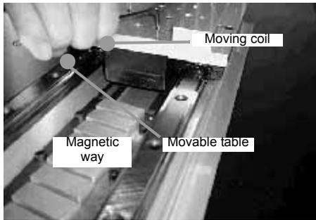
Maintain the following air gaps when installing. Make sure that the moving coil and magnetic way do not interfere with each other during the stroke.
