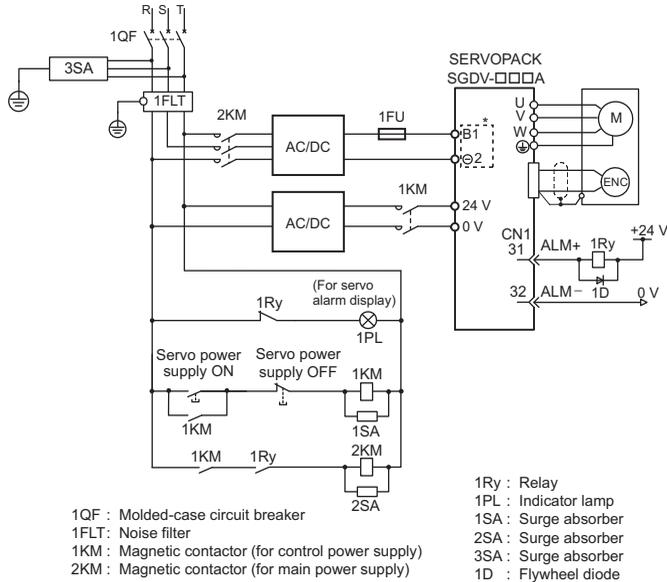
\* The terminal names differ depending on the SERVOPACK model. Refer to (2) *Main Circuit and Control Power Inputs*.
