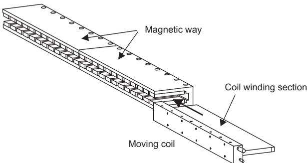
The relationship between the dimensions and positioning between the moving coil's coil winding section and magnetic ways's magnets is shown here. Maintain the following air gaps when installing. Make sure that the moving coil and magnetic way do not interfere with each other during the stroke.
