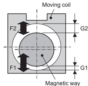
The figure shown on the right is an example in which a non-uniform gap occurs. Actually, magnetic attraction may be generated and extended in all directions because of an assembling error or other reasons.
