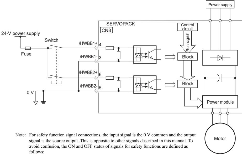
Note: For safety function signal connections, the input signal is the 0 V common and the output signal is the source output. This is opposite to other signals described in this manual. To avoid confusion, the ON and OFF status of signals for safety functions are defined as follows:
