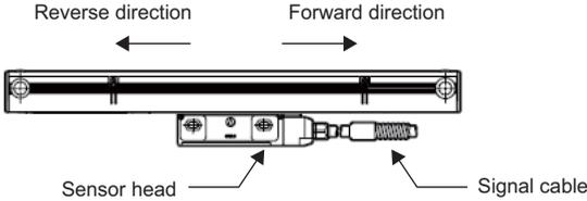
When installed as shown in the diagram on the left, operation is performed in the forward direction when the sensor head is moved to the right.
