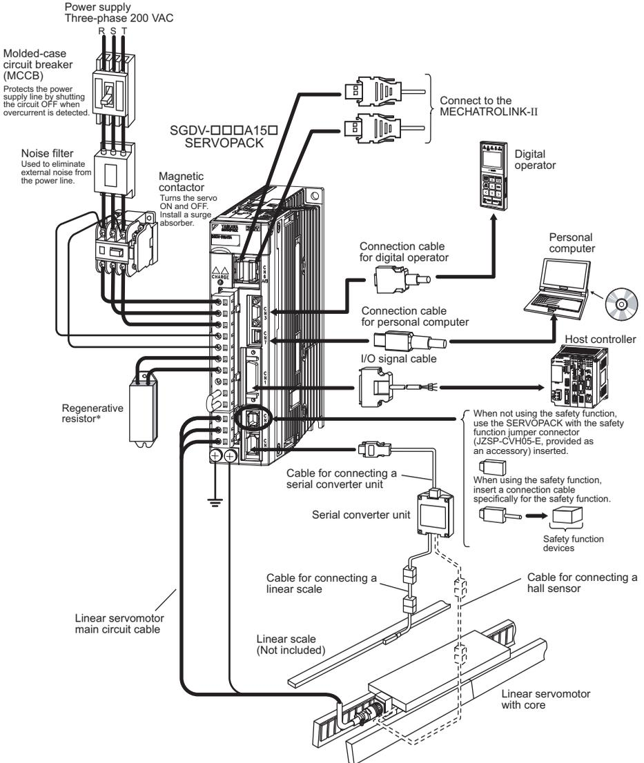
\* Before connecting an external regenerative resistor to the SERVOPACK, refer to 3.4 Connecting Regenerative Resistors.
