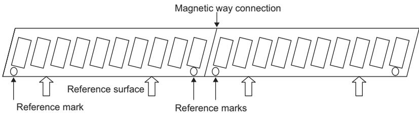
3. While placing the magnetic way on the machine base reference surface, secure it with bolts.
