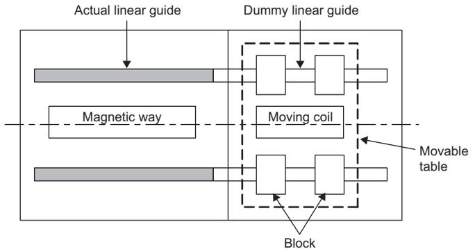
2. Insert a thin nonmagnetic (preferably resin) sheet (approximately 0.5-mm thick) in the air gap between the moving coil and magnetic way. Then, and move the moving coil toward the magnetic way.
