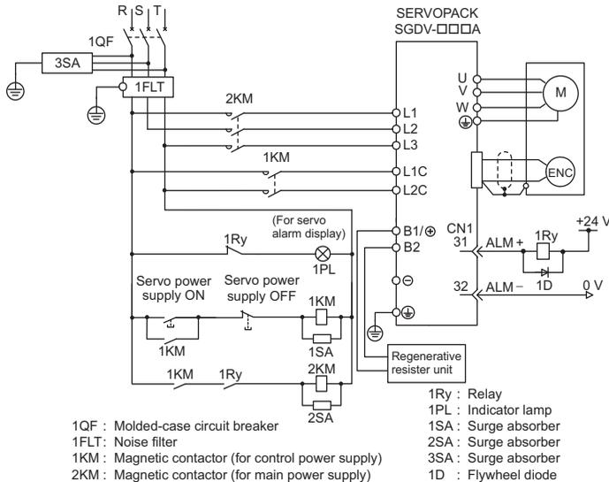
Note: For M-II model, M-III model, and command option attachable type SERVOPACKS, the pin number of ALM+ terminal is CN1-3, and that of ALM- terminal is CN1-4.
