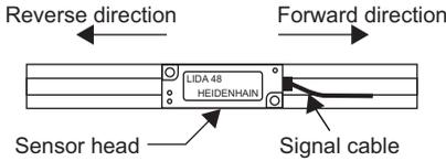
When installed as shown in the diagram on the left, operation is performed in the forward direction when the sensor head is moved to the right.
