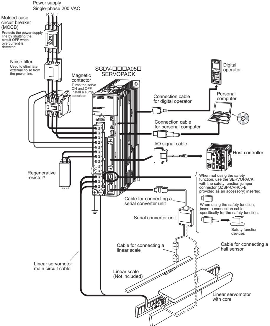
\* Before connecting an external regenerative resistor to the SERVOPACK, refer to 3.4 Connecting Regenerative Resistors.
