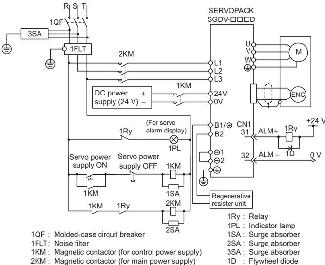
Note: For M-II model, M-III model, and command option attachable type SERVOPACKs, the pin number of ALM+ terminal is CN1-3, and that of ALM- terminal is CN1-4.
